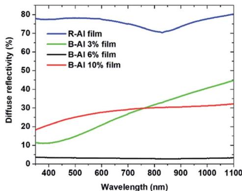
Fig. 4 Diffuse reflectivity from R-Al and B-Al films as a function of the N<sub>2</sub> percent used during the deposition step.
