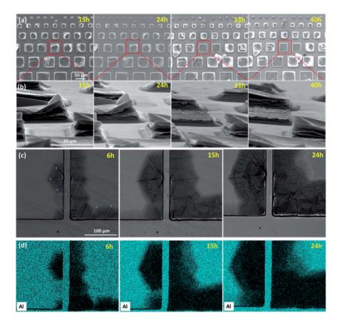
Fig. 2 (a) SEM images of  $V_2$ AlC pillars with various sizes and (b) corresponding  $82^{\circ}$  tilted views of red dotted square in images in (a) as a function of HF etching time. (c) SEM images and (d) EDS mapping of Al atom lines, of a 500  $\mu$ m sized pillar as a function of HF etching time. Arrows in (c) indicate preferred etching directions, tracing in some cases hexagon-like structures.
