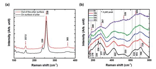
Fig. 4 Representative Raman spectra measured (a) at the top surface of an un-etched V<sub>2</sub>AlC pillar and in the trench area exposed to a chlorine RIE etching process, (b) on a  $V_2CT_z$  area etched by HF for 6 h, 15 h, 24 h, 33 h and 40 h.
