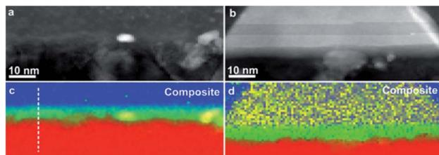
Fig. 6 (a and b) HAADF STEM images of two interfacial areas between the Si substrate and the carbon layer in NCD-1; (c and d) superposition of EELS maps of K-edges of Si (blue), C (red), O (green), and Ni L-edge (yellow). The white dashed line in (c) marks the position of the profile shown in Fig. 8a.
