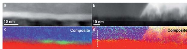
Fig. 7 (a and b) HAADF STEM images of two interfacial areas between the Si substrate and the carbon layer in NCD-2; (c and d) superposition of EELS maps of K-edges of Si (blue), C (red), O (green), and Ni L-edge (yellow). The white dashed line in (d) marks the position of the profile shown in Fig. 8b.
