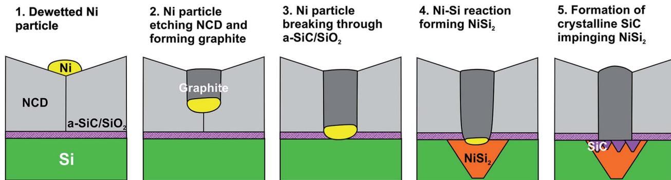
Fig. 9 Scheme of the Ni–C, Ni–Si and Si–C solid-state reactions leading to NiSi<sub>2</sub> and SiC formation at the initial Si/NCD interface in NCD-2.
