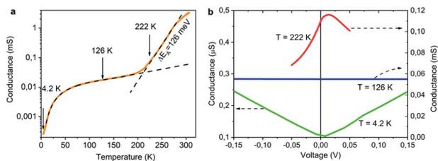
Fig. 11 (a)  $G(T)$  of NCD-2 plotted in a semi-logarithmic scale. (b) Voltage dependence of conductance measured at  $T = 4.2$  K (green), 126 K (blue), and 222 K (red) showing different conductance regimes.
