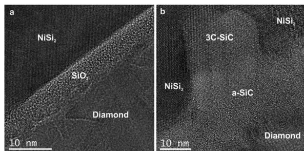
Fig. 5 HRTEM images of the phases occurring near the base of NiSi<sub>2</sub> pyramids formed in samples (a) NCD-1 and (b) NCD-2.
