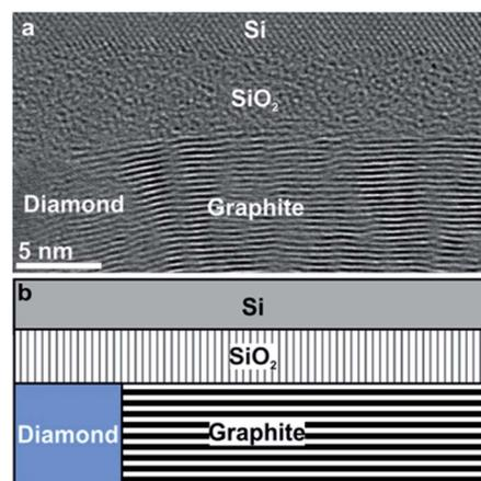
Fig. 2 HRTEM image of NCD-1 shows in cross section retained diamond, catalytically converted graphite and the Si substrate with its native  $\text{SiO}_2$  layer. (a) Graphite is grown with the (0001) planes almost perpendicular to the diamond surface and parallel to the  $\text{Si}/\text{SiO}_2$  interface. (b) Sketch of the diamond/graphite- $\text{SiO}_2/\text{Si}$  configuration seen in (a).
