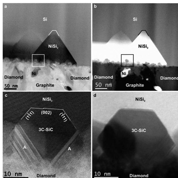
**Fig. 4** Cross-sectional STEM images of NCD-2. (a) BF and (b) HAADF images show the retained NCD/graphite layer with some embedded Ni nanoparticles below and Si with embedded NiSi<sub>2</sub> pyramids and additional layer consisting of 10–30 nm sized grains above the interface. (c) BF and (d) corresponding HAADF image of a nanocrystal with a 3C-SiC cubic phase.
