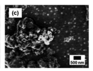
Fig. 6 Top view SEM micrographs of SiNCs/PTB7 photoactive layer: (a) as-etched SiNCs; (b) low-defect SiNCs (200 °C annealing); (c) high-defect SiNCs (400 °C annealing).
