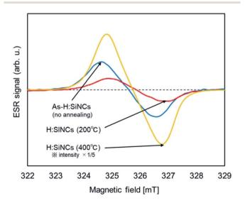
Fig. 3 ESR spectra of SiNCs before and after thermal annealing; As-H:SiNCs (no annealing), H:SiNCs (200  $^{\circ}$ C for 1 hour) and H:SiNCs (200  $^{\circ}$ C for 1 hour).
