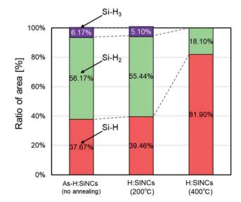
Fig. 4 Ratio of hydrogen groups on SiNC surface.
