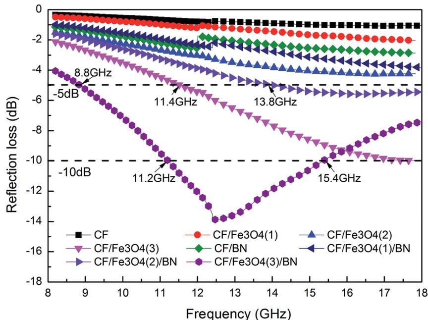
Fig. 11 EM wave absorption properties of CF, CF/BN, CF/Fe<sub>3</sub>O<sub>4</sub>(1), CF/Fe<sub>3</sub>O<sub>4</sub>(2), CF/Fe<sub>3</sub>O<sub>4</sub>(3), CF/Fe<sub>3</sub>O<sub>4</sub>(1)/BN, CF/Fe<sub>3</sub>O<sub>4</sub>(2)/BN, and CF/Fe<sub>3</sub>O<sub>4</sub>(3)/BN composites.
