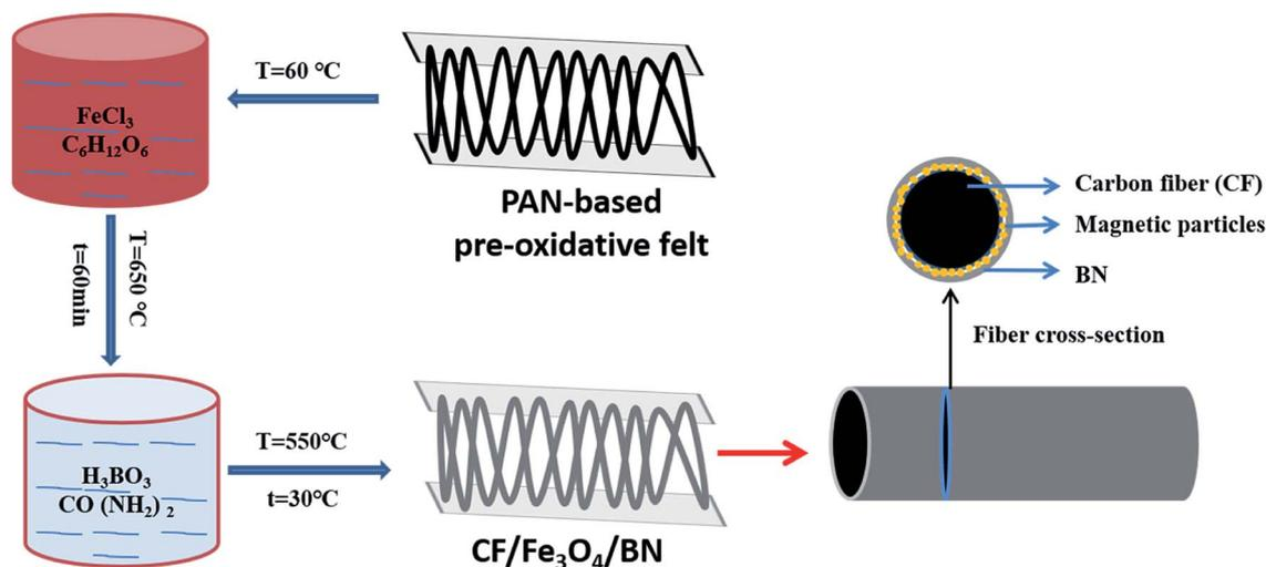
Fig. 1 Preparation process for CF/ $\text{Fe}_3\text{O}_4$ /BN composites.
