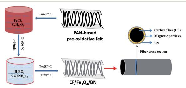
Fig. 1 Preparation process for CF/Fe<sub>3</sub>O<sub>4</sub>/BN composites.
