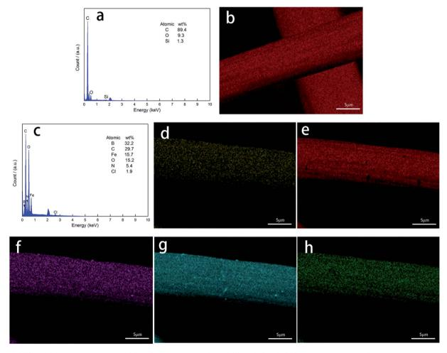
Fig. 4 EDS (a) and SEM topography maps (b) of CF for elements C; EDS (c) of CF/Fe $_3$ O $_4$ (3)/BN composites and SEM topography maps of CF/Fe $_3$ O $_4$ (3)/BN composites for elements (d) B, (e) C, (f) Fe, (g) O, and (h) N.
