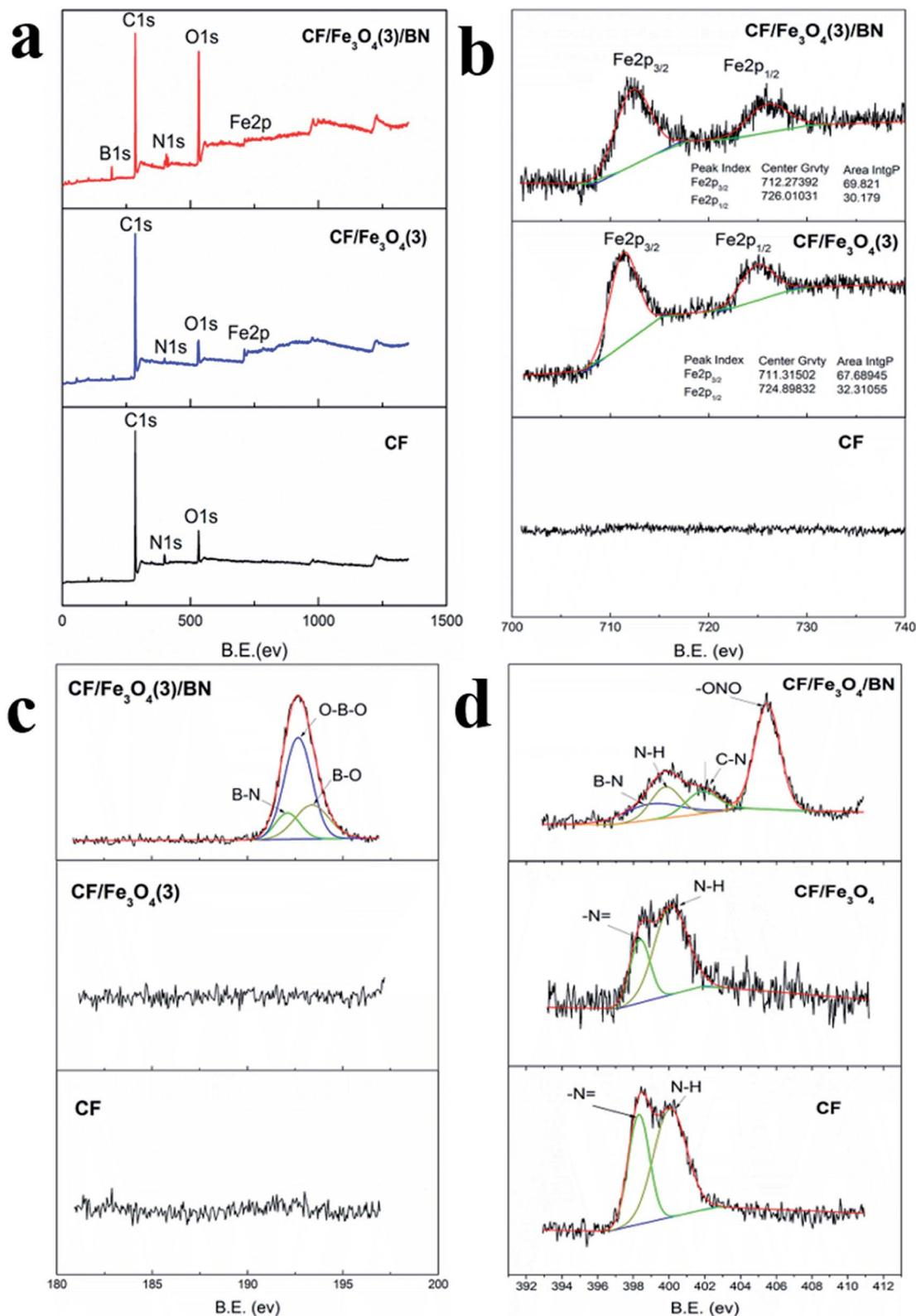
Fig. 5 XPS spectra: (a) wide scan, and (b) Fe2p, (c) B1s, and (d) N1s spectra of CF, CF/Fe<sub>3</sub>O<sub>4</sub>(3) and CF/Fe<sub>3</sub>O<sub>4</sub>(3)/BN composites.
