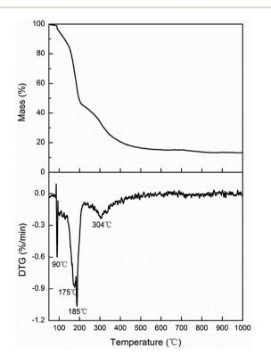
Fig. 7 Thermogravimetry (TG) and derivative thermogravimetric (DTG) curves of boric acid and urea.
