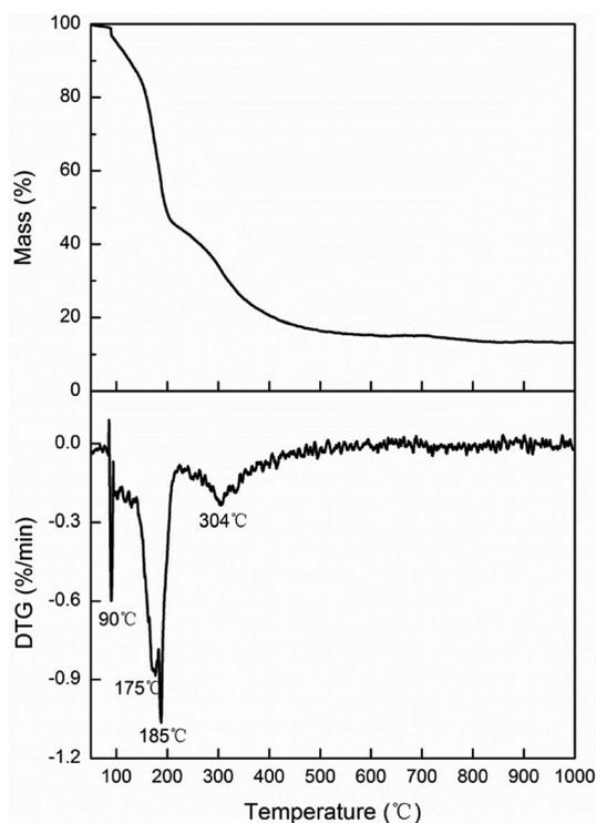
**Fig. 7** Thermogravimetry (TG) and derivative thermogravimetric (DTG) curves of boric acid and urea.
