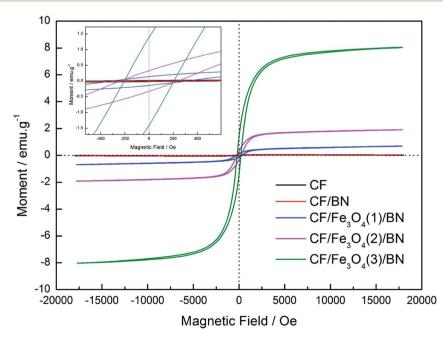
Fig. 6 Magnetic hysteresis loops of CF, CF/BN, CF/Fe<sub>3</sub>O<sub>4</sub>(1)/BN, CF/Fe<sub>3</sub>O<sub>4</sub>(2)/BN and CF/Fe<sub>3</sub>O<sub>4</sub>(3)/BN composites.
