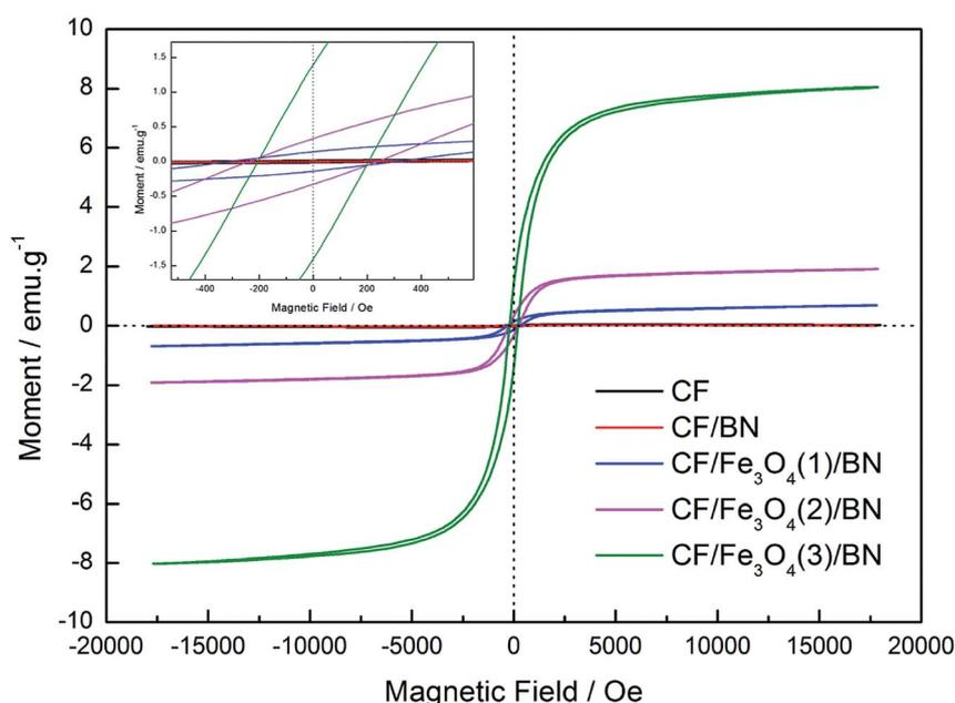
Fig. 6 Magnetic hysteresis loops of CF, CF/BN, CF/Fe<sub>3</sub>O<sub>4</sub>(1)/BN, CF/Fe<sub>3</sub>O<sub>4</sub>(2)/BN and CF/Fe<sub>3</sub>O<sub>4</sub>(3)/BN composites.
