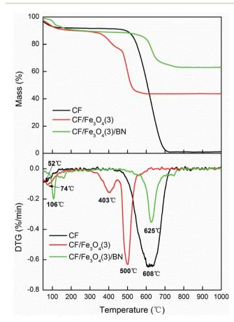
Fig. 8 TG and DTG curves of CF, CF/Fe<sub>3</sub>O<sub>4</sub>(3) and CF/Fe<sub>3</sub>O<sub>4</sub>(3)/BN.
