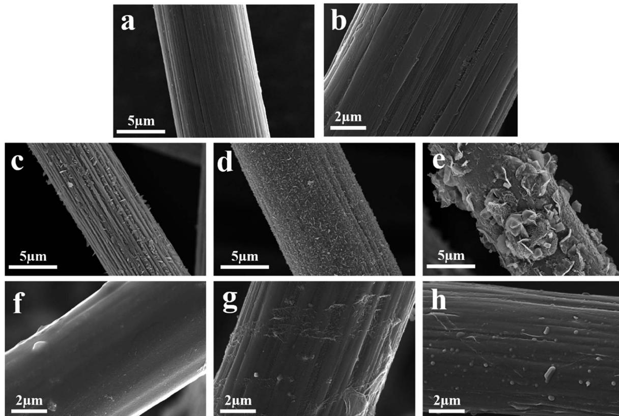
Fig. 3 SEM images of (a) CF, (b) CF/BN, (c) CF/Fe<sub>3</sub>O<sub>4</sub>(1), (d) CF/Fe<sub>3</sub>O<sub>4</sub>(2), (e) CF/Fe<sub>3</sub>O<sub>4</sub>(3), (f) CF/Fe<sub>3</sub>O<sub>4</sub>(1)/BN, (g) CF/Fe<sub>3</sub>O<sub>4</sub>(2)/BN, and (h) CF/Fe<sub>3</sub>O<sub>4</sub>(3)/BN.
