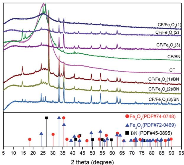
Fig. 2 XRD profiles for CF, CF/Fe<sub>3</sub>O<sub>4</sub>, and CF/Fe<sub>3</sub>O<sub>4</sub>/BN composites.
