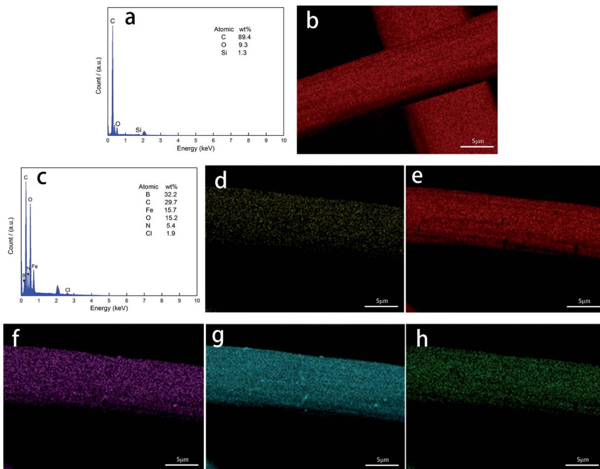
Fig. 4 EDS (a) and SEM topography maps (b) of CF for elements C; EDS (c) of CF/ $\text{Fe}_3\text{O}_4$ (3)/BN composites and SEM topography maps of CF/ $\text{Fe}_3\text{O}_4$ (3)/BN composites for elements (d) B, (e) C, (f) Fe, (g) O, and (h) N.
