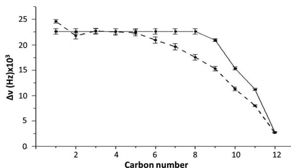
Fig. 3 Comparison of  $\Delta\nu_{\text{Q}}$  between experiment (system 2) (continuous line) and MD simulations (Box 2) (dashed line) as a function of the carbon number. Error bars represent the standard deviation. See Table S1† for exact numbers.
