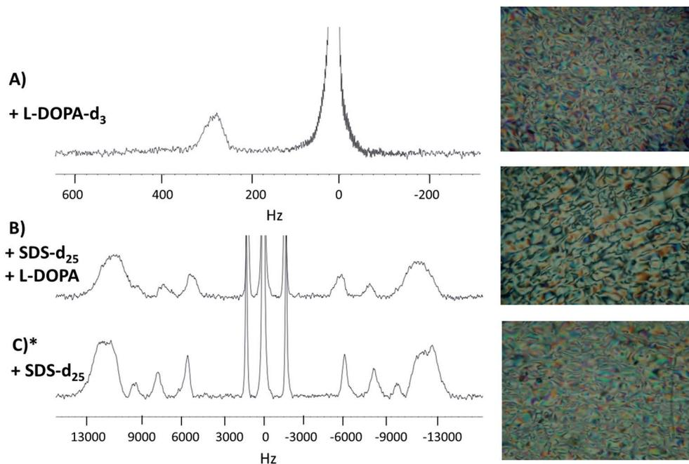
Fig. 2  $^2\text{H}$ -NMR spectra and the PLM textures. Panel (A), L-DOPA- $\text{d}_3$  in system 2. Panel (B), SDS- $\text{d}_{25}$  in system 2. Panel (C), SDS- $\text{d}_{25}$  in system 1. \* System 1 spectrum and PLM texture were obtained in a previous work and are reproduced with permission from ref. 27.
