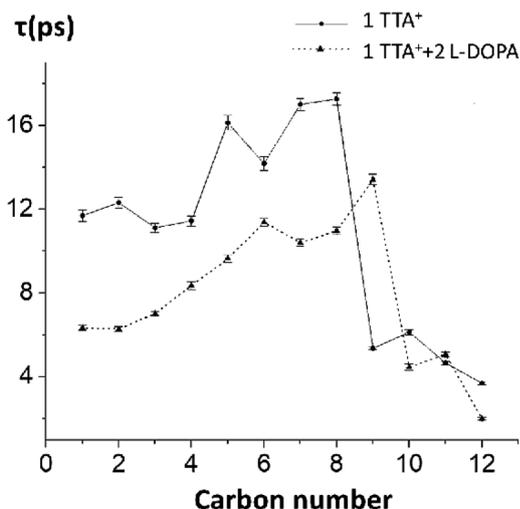
Fig. 6 Representative  $\tau$  for the mono-exponential decay of autocorrelation function of  $S_{CH}$  for each C-H bond in TTA<sup>+</sup>, with and without L-DOPA. These values were obtained from the simulation of the box containing only water, TTA<sup>+</sup> and a Cl<sup>-</sup>.
