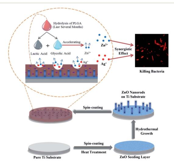
Fig. 6 Schematic illustration of the fabrication process of poly(lactic-co-glycolic acid)/Ag/ZnO nanorods composite coating.<sup>131</sup>
