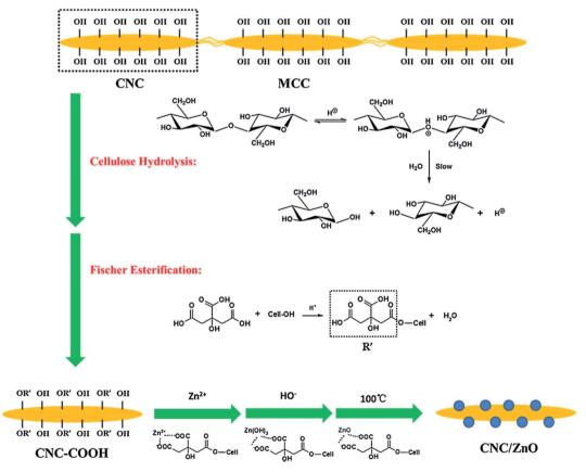
Fig. 9 The preparation route of cellulose nanocrystal/zinc oxide (CNC/ZnO) nanohybrids.<sup>164</sup>
