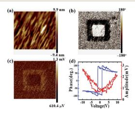
Fig. 2 (a) Topological, (b) PFM phase and (c) amplitude images of the of BEFO film after applying +10 V (inner square 0.6  $\mu$ m  $\times$  0.6  $\mu$ m) and -10 V (outer square 1.0  $\mu$ m  $\times$  1.0  $\mu$ m) bias at the center of the region, respectively. (d) PFM phase and amplitude hysteresis loops.
