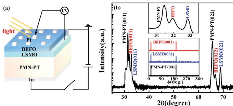
Fig. 1 (a) Schematic of Pt/BEFO/LSMO/PMN-PT heterostructures. (b) XRD  $\theta$ – $2\theta$  scan of the heterostructures, and the inset (up) is the expanded view near BEFO (011) diffraction peak, the inset (down) is  $\phi$ –scan of the BEFO (011) and NSTO (011) planes.
