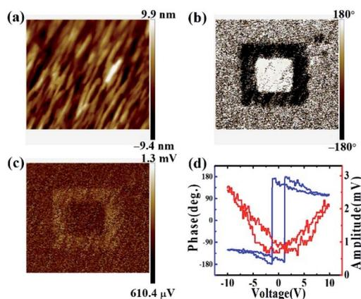
Fig. 2 (a) Topological, (b) PFM phase and (c) amplitude images of the of BEFO film after applying  $+10 \text{ V}$  (inner square  $0.6 \mu\text{m} \times 0.6 \mu\text{m}$ ) and  $-10 \text{ V}$  (outer square  $1.0 \mu\text{m} \times 1.0 \mu\text{m}$ ) bias at the center of the region, respectively. (d) PFM phase and amplitude hysteresis loops.
