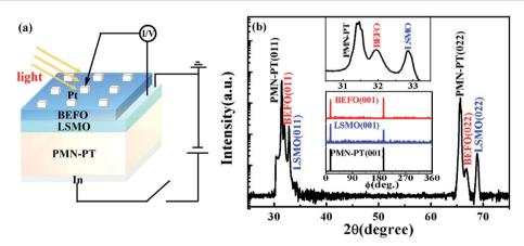
Fig. 1 (a) Schematic of Pt/BEFO/LSMO/PMN-PT heterostructures. (b) XRD  $\theta$ -2 $\theta$  scan of the heterostructures, and the inset (up) is the expanded view near BEFO (011) diffraction peak, the inset (down) is  $\phi$ -scan of the BEFO (011) and NSTO (011) planes.
