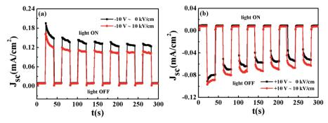
Fig. 5 (a and b)  $J_{sc}$  switching of the BEFO film in the dark and under light illumination by switching the polarization.  $J_{sc}$  as a function of time upon turning the light on and off for the Pt/BEFO/LSMO/PMN-PT device with and without the application of an electric field of  $\pm 10$  kV cm<sup>-1</sup> to the PMN-PT substrate, where the BEFO film was in the  $P_r^+$  and  $P_r^-$  states, respectively.
