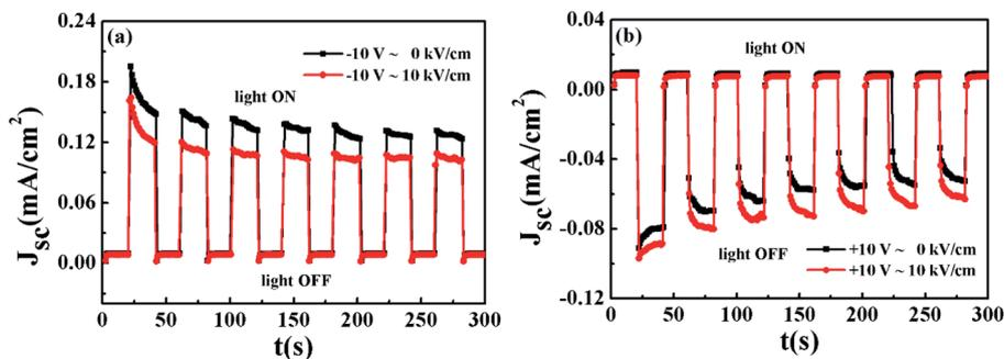
Fig. 5 (a and b)  $J_{sc}$  switching of the BEFO film in the dark and under light illumination by switching the polarization.  $J_{sc}$  as a function of time upon turning the light on and off for the Pt/BEFO/LSMO/PMN-PT device with and without the application of an electric field of  $+10 \text{ kV cm}^{-1}$  to the PMN-PT substrate, where the BEFO film was in the  $P_r^+$  and  $P_r^-$  states, respectively.
