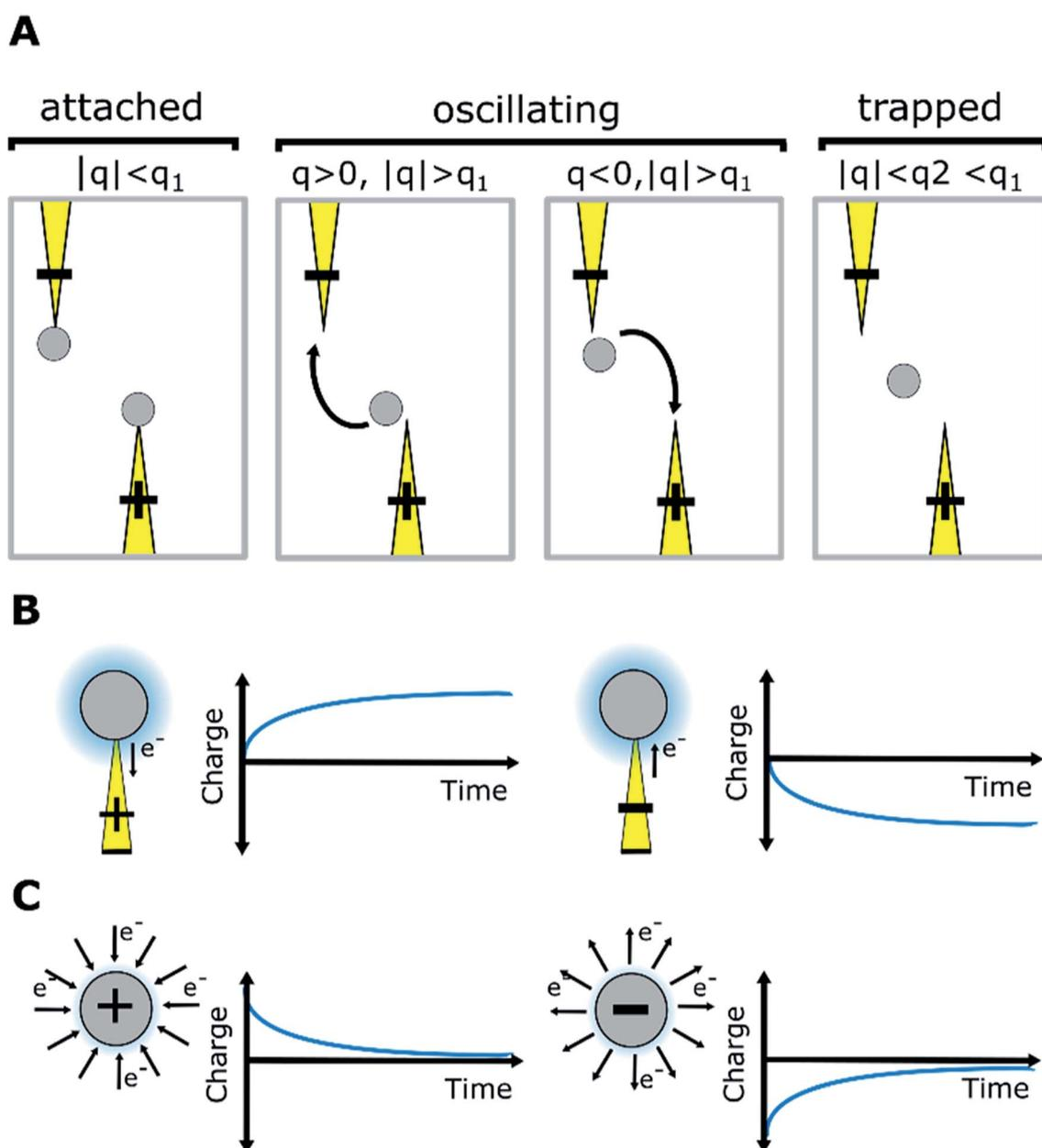
Fig. 6 (A) Microparticle trajectory indicates the sign and magnitude of charge;  $q$  is the particle instant charge,  $q_1$  and  $q_2$  are charge thresholds. (B) Microparticle charging. (C) Microparticle charge relaxation.
