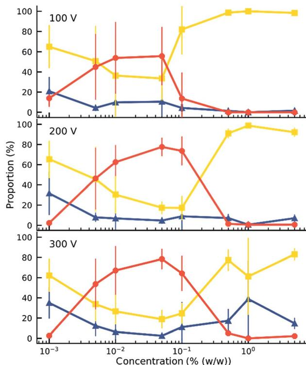
Fig. 3 Proportion of trapped ( $\blacktriangle$ ), oscillating ( $\bullet$ ), and attached ( $\blacksquare$ ) microparticles in a sample according to the surfactant concentration and applied voltage. The solid lines are guides to the eye. Error bars indicate standard deviation.
