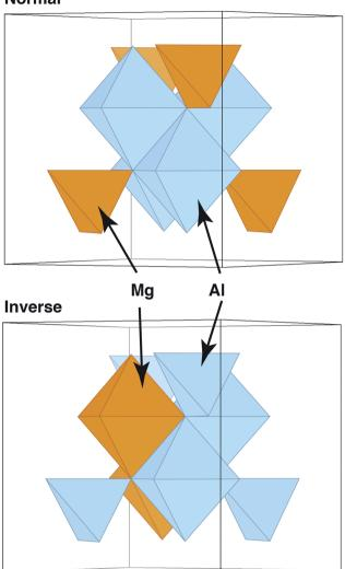
Fig. 1 Schematic representation of the difference between a normal and an inverse spinel structure. In the normal structure, the tetrahedral polyhedra are occupied by the A cation (Mg in  $MgAl_2O_4$ ) while the octahedral positions are filled with Al. In the inverse structure, all tetrahedral positions are filled by the B cation (Al if  $MgAl_2O_4$  were to be fully inverse) while half of the octahedral positions are occupied by Mg.
