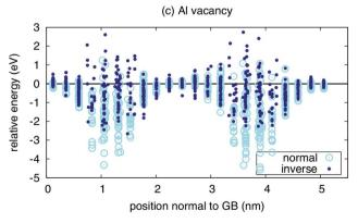
Fig. 4 Energetics of vacancies near both the ideal (normal) and minimized (inverse)  $\Sigma 3(111)$  grain boundary for three types of vacancies: (a) oxygen, (b) magnesium, and (c) aluminum.
