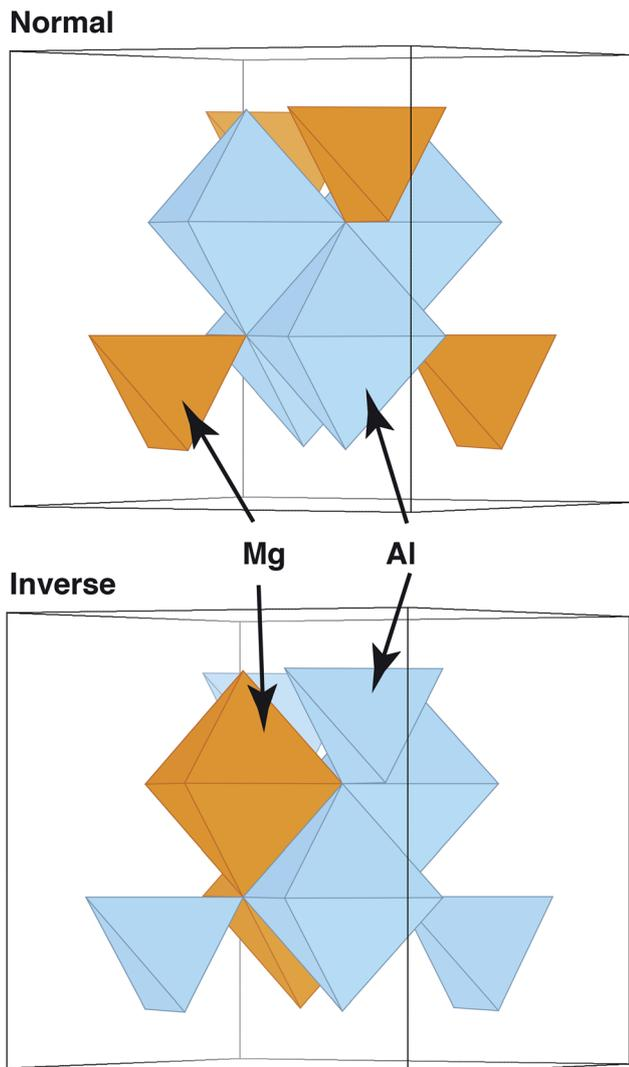
Fig. 1 Schematic representation of the difference between a normal and an inverse spinel structure. In the normal structure, the tetrahedral polyhedra are occupied by the A cation (Mg in  $\text{MgAl}_2\text{O}_4$ ) while the octahedral positions are filled with Al. In the inverse structure, all tetrahedral positions are filled by the B cation (Al if  $\text{MgAl}_2\text{O}_4$  were to be fully inverse) while half of the octahedral positions are occupied by Mg.
