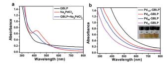
Fig. 1 (a) UV-Vis spectra of GBLP,  $Na_2PdCl_4$ , GBLP +  $Na_2PdCl_4$ , (b) UV-Vis spectra and photos of 5  $\mu$ M of  $Pd_n$ -GBLP NPs.
