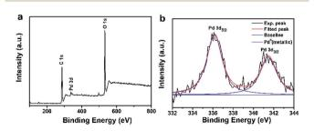
Fig. 3 (a) XPS spectrum of Pd $_{91}$ -GBLP NPs and (b) high-resolution spectrum of the Pd 3d.
