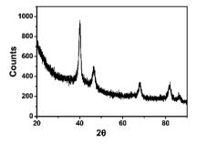
Fig. 4 The XRD pattern of Pd<sub>91</sub>-GBLP NPs.
