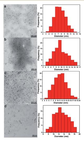
Fig. 2 TEM images and corresponding size distribution histograms of (a)  $Pd_{41}$ -GBLP, (b)  $Pd_{68}$ -GBLP, (c)  $Pd_{91}$ -GBLP and (d)  $Pd_{137}$ -GBLP.
