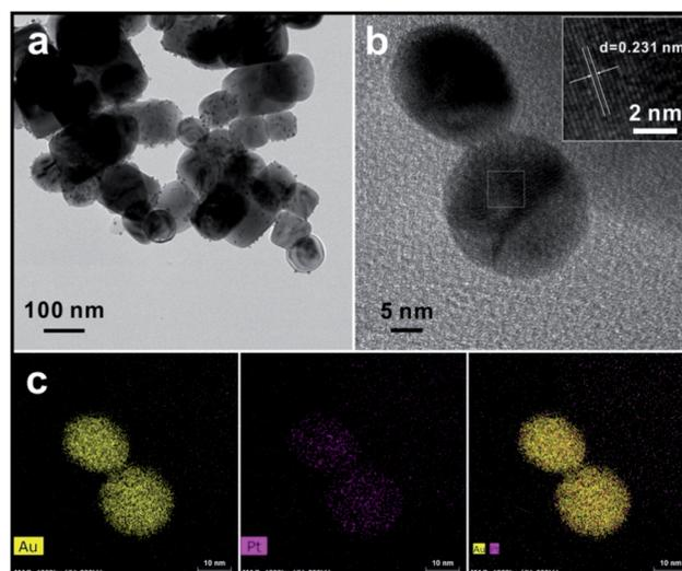
Fig. 3 (a and b) TEM images of Au/Pt bimetallic NPs on the surface of BTO with different magnification, and the image inset in (b) is the HRTEM image of Au/Pt bimetallic NPs with measured lattice distance. (c) EDS mapping images of Au/Pt bimetallic NPs on the surface of BTO. Colored pixels indicate where the element was detected above background.
