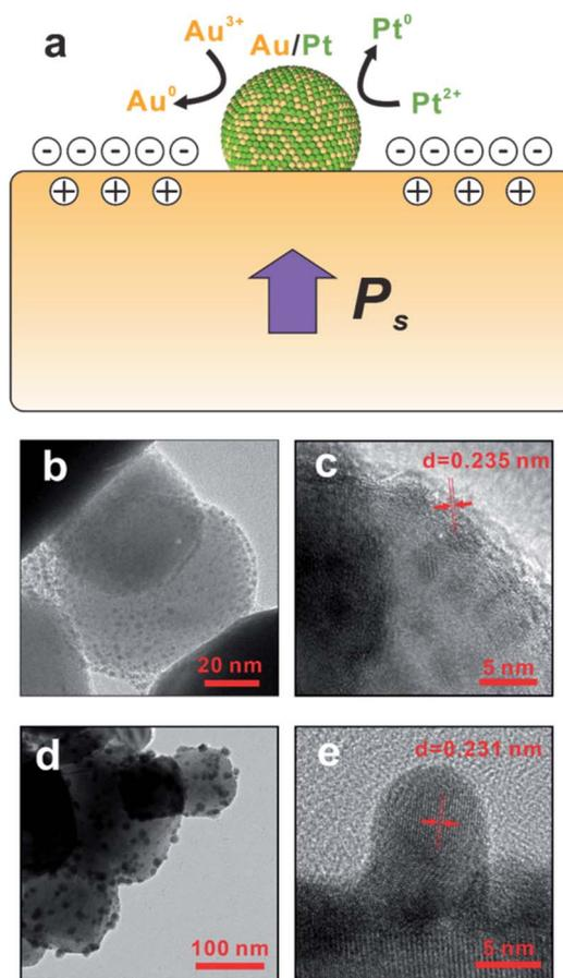
Fig. 4 (a) Scheme illustration of the pyro-catalytic reaction mechanism, *i.e.*, the cold-hot alternation excitation of a pyroelectric material and the subsequent redox reaction on the surface. (b) low-magnified TEM image of the growth of the particles at early stage; (c) early-stage HRTEM image of the particle with lattice spacing. (d) low-magnified TEM image of the growth of the Au/Pt NPs at late stage; (e) late-stage HRTEM image of the Au/Pt NPs with lattice spacing.
