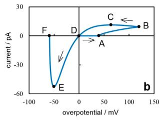
Fig. 4 Dependence of the nanocluster radius on the overpotential (a) and the cyclic voltammogram (b). Calculation parameters are reported in the text. The points mentioned in the text are marked on the cyclic voltammogram.
