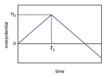
$\label{eq:Fig. 3} \mbox{ Scheme of the time dependence of overpotential in cyclic voltammetry.}$
