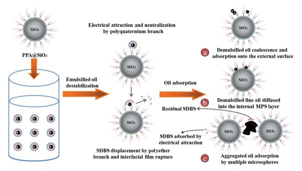
Fig. 5 Schematic diagram of proposed oil adsorption mechanism of PPA@SiO<sub>2</sub> towards the O/W emulsion (a) oil coalescence, (b) oil diffusion, and (c) oil-loaded microspheres aggregation.
