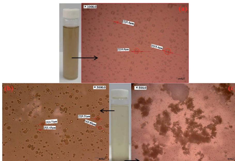
Fig. 3 Micro morphologies of oil droplets in (a) simulated ASP flooding produced water; (b) 1.0 g L<sup>-1</sup> PPA@SiO<sub>2</sub> treated produced water and (c) oil-loaded PPA@SiO<sub>2</sub> microspheres.
