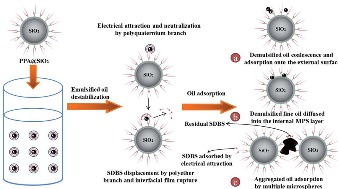
Fig. 5 Schematic diagram of proposed oil adsorption mechanism of PPA@SiO<sub>2</sub> towards the O/W emulsion (a) oil coalescence, (b) oil diffusion, and (c) oil-loaded microspheres aggregation.
