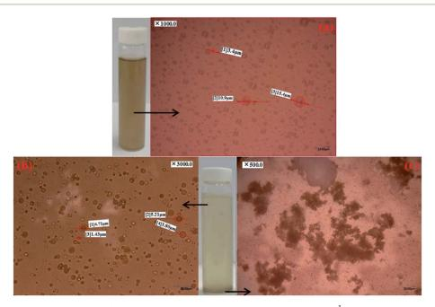
Fig. 3 Micro morphologies of oil droplets in (a) simulated ASP flooding produced water; (b) 1.0 g L<sup>-1</sup> PPA@SiO<sub>2</sub> treated produced water and (c) oil-loaded PPA@SiO2 microspheres.
