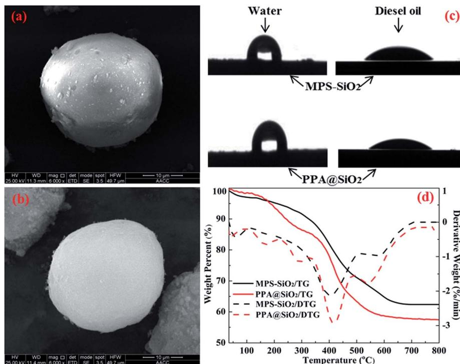
Fig. 2 SEM images of (a) MPS-SiO<sub>2</sub> and (b) PPA@SiO<sub>2</sub>; (c) contact angles and (d) TG/DTG curves for the MPS-SiO<sub>2</sub> and PPA@SiO<sub>2</sub> microspheres.
