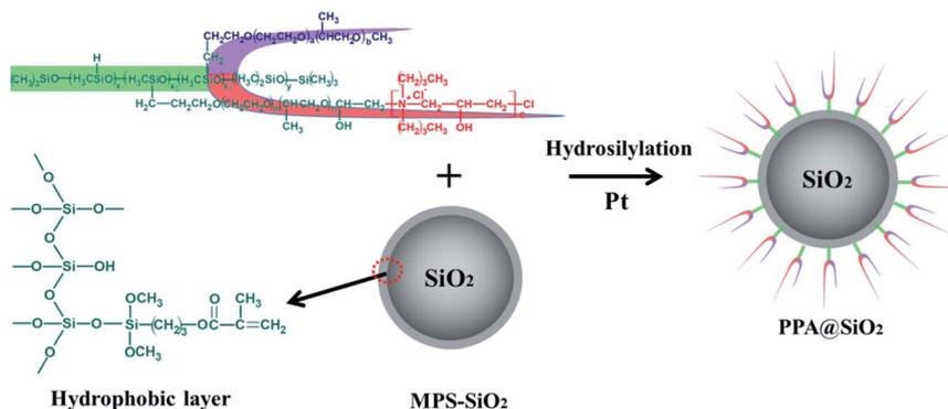
Fig. 1 Preparation of the functional PPA@SiO<sub>2</sub> microsphere.
