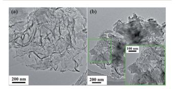
Fig. 1 TEM images of  $g-C_3N_4-Ns$  (a) and  $g-C_3N_4-Ns-PEI-GA@CALB$  (b).
