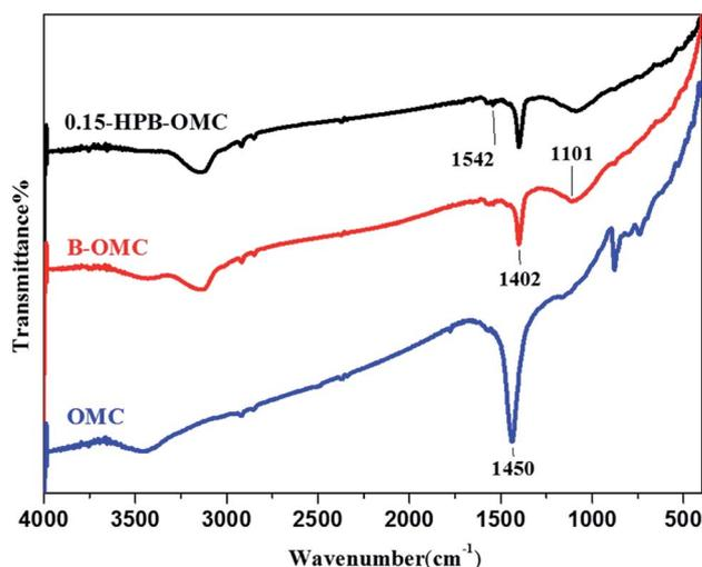
Fig. 2 FT-IR spectra of OMC, B-OMC, and 0.15-HPB-OMC.
