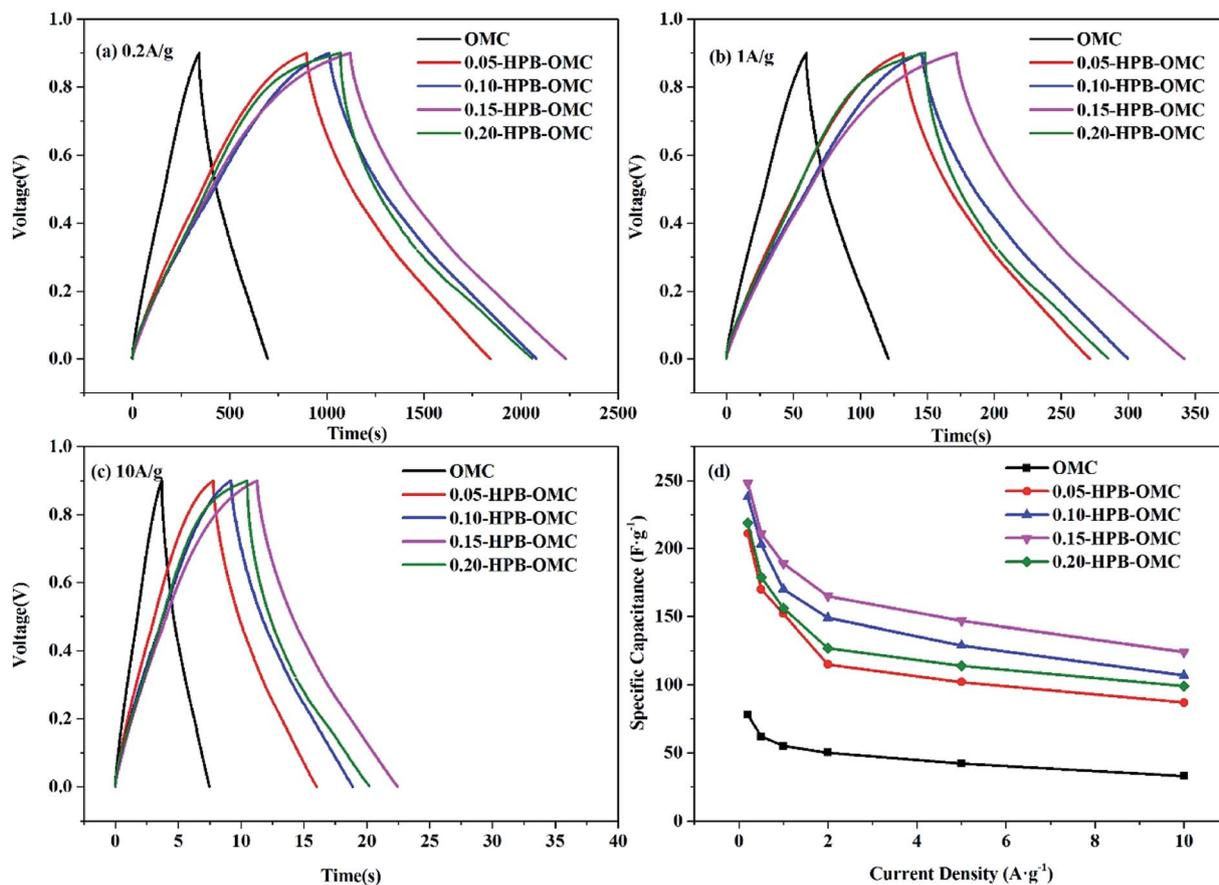
Fig. 7 GCD curves of the HPB-OMCs at a current density of 0.2 A g<sup>-1</sup> (a), 1 A g<sup>-1</sup> (b), 10 A g<sup>-1</sup> (c), and specific capacitance of HPB-OMCs at different current density (d).
