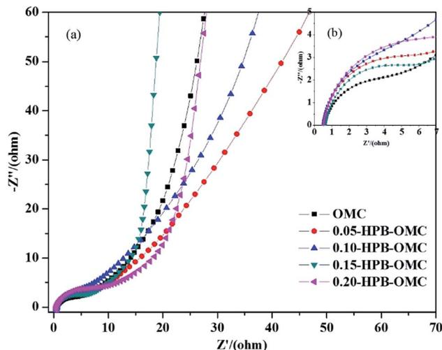
Fig. 9 (a) Nyquist plots of HPB-OMCs and (b) the enlargement at high frequency region.
