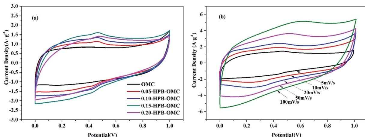
Fig. 8 CV curves of various HPB-OMCs at a scan rate of 5 mV s<sup>-1</sup> (a) and CV curves of 0.15-HPB-OMC at different scan rate (b).
