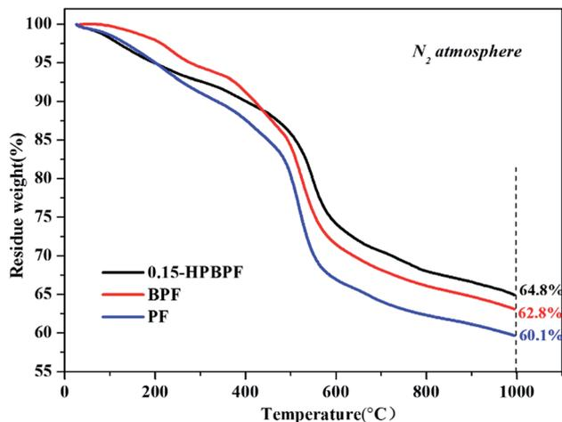
Fig. 1 Thermogravimetric analysis curves of the PF, BPF, and 0.15-HPBPF with a heating rate of 10 °C min<sup>-1</sup> in N<sub>2</sub>.
