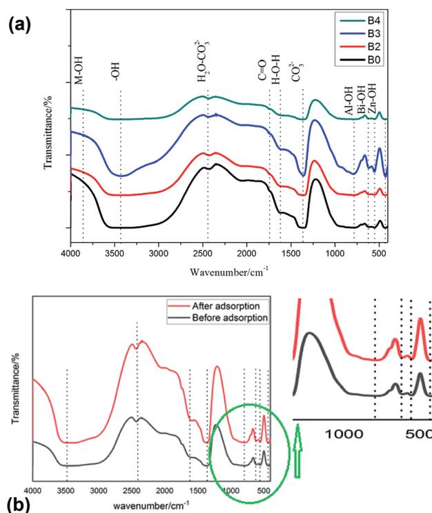
Fig. 2 (a) FTIR spectra of ZnAl-LDH (B0),  $\text{Bi}_{0.2}\text{ZnAl}_{0.8}$ -LDH (B2),  $\text{Bi}_{0.3}\text{ZnAl}_{0.7}$ -LDH (B3) and  $\text{Bi}_{0.4}\text{ZnAl}_{0.6}$ -LDH (B4). (b) FTIR spectra of BiZnAl-LDH (Bi/Zn/Al=0.4 : 3 : 0.6) before and after adsorption.
