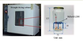
Fig. 1 Schematic of the device for the iodine adsorption experiments in static air.
