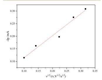
Fig. 4 Cathodic peak current of cyclic voltammograms at 333 K under different scan rates.
