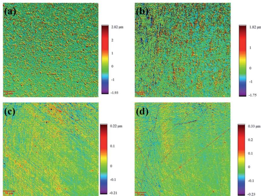
Fig. 9 Surface topography of the nickel coating electrodeposited in IL with different water concentration at 363 K: (a) 5 wt%, (b) 10 wt%, (c) 20 wt%, (d) 30 wt%.
