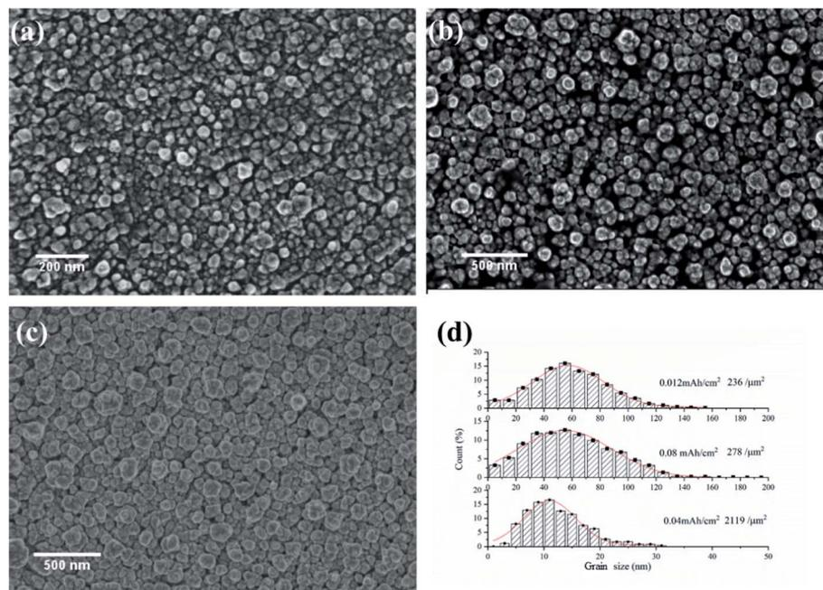
Fig. 5 (a–c) SEM images of Ni coatings formed on copper substrate under potentiostatic deposition at  $-0.6$  V (vs. Ag) and 363 K for a total capacity of  $0.04$  mA h  $\text{cm}^{-2}$ ,  $0.08$  mA h  $\text{cm}^{-2}$  and  $0.12$  mA h  $\text{cm}^{-2}$  respectively. (d) Histogram of grain size obtained from (a–c).
