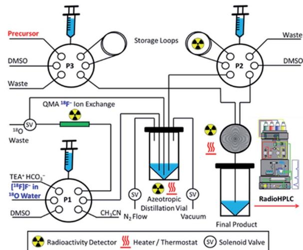
Fig. 9 Automated synthesis module for the azeotropic drying of cyclotron generated  $^{18}\text{F}$ fluoride and subsequent microfluidic set-up for the rhenium(i) complexation–dissociation reactions under varying reaction environments.
