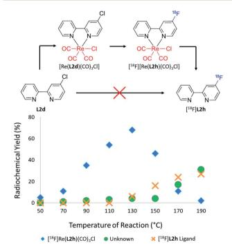
Fig. 4 RCYs of [18F][Re(L2h)(CO)<sub>3</sub>Cl] (blue diamonds), [18F]L2h (orange crosses) and an unknown by-product (green circles) plotted as a function of the reaction temperature for the [18F]fluoride labelling of the para substituted [Re(CO)<sub>3</sub>(L2d)Cl] complex. [18F]L2h was unable to be synthesised from L2d unless mediated by rhenium(ı) complexation as per the above scheme.
