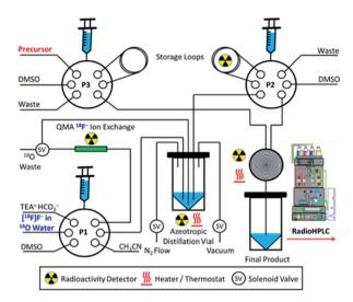
Fig. 9 Automated synthesis module for the azeotropic drying of cyclotron generated [<sup>18</sup>F]fluoride and subsequent microfluidic set-up for the rhenium(i) complexation–dissociation reactions under varying reaction environments.
