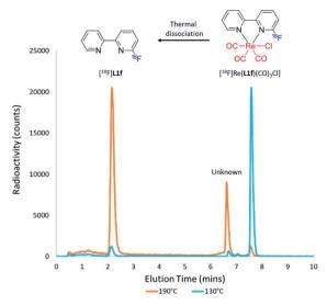
Fig. 2 Radiochromatogram profiles for the fluorine-18 labelling of [Re(L1b)(CO)<sub>3</sub>Cl] at 130 °C (blue trace) and 190 °C (orange trace). At 130 °C [18F][Re(L1f)(CO)<sub>3</sub>Cl] (7.6 min) forms in the greatest yield, whereas at 190 °C the complex dissociates to form the otherwise unobtainable [18F]L1f ligand (2.2 min) alongside an unknown byproduct (6.6 min).
