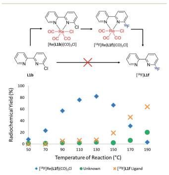
Fig. 3 [18F]Fluoride substitution in the ortho position of [Re(L1b)(CO)<sub>3</sub>Cl] which afforded [<sup>18</sup>F][Re(L1f)(CO)<sub>3</sub>Cl] (blue diamonds). Thermal decomplexation led to the subsequent formation of [18F]L1f (orange crosses) and an unknown by-product (green circles) with the RCYs plotted as a function of reaction temperature. [18F]L1f was unable to be synthesised from L1b without first complexing to a rhenium(1) centre
