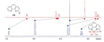
Fig. 6 Example of the downfield chemical shifts in  $^1\text{H-NMR}$  aromatic signals observed when complexing L2b (top, red) with [Re(CO) $_5$ Cl] to form [Re(L2b)(CO) $_3$ Cl] (bottom, blue). The shifts suggest electron withdrawal from the  $\pi$ -aromatic system which likely facilitates nucleophilic substitution for [ $^{18}$ F]fluoride.
