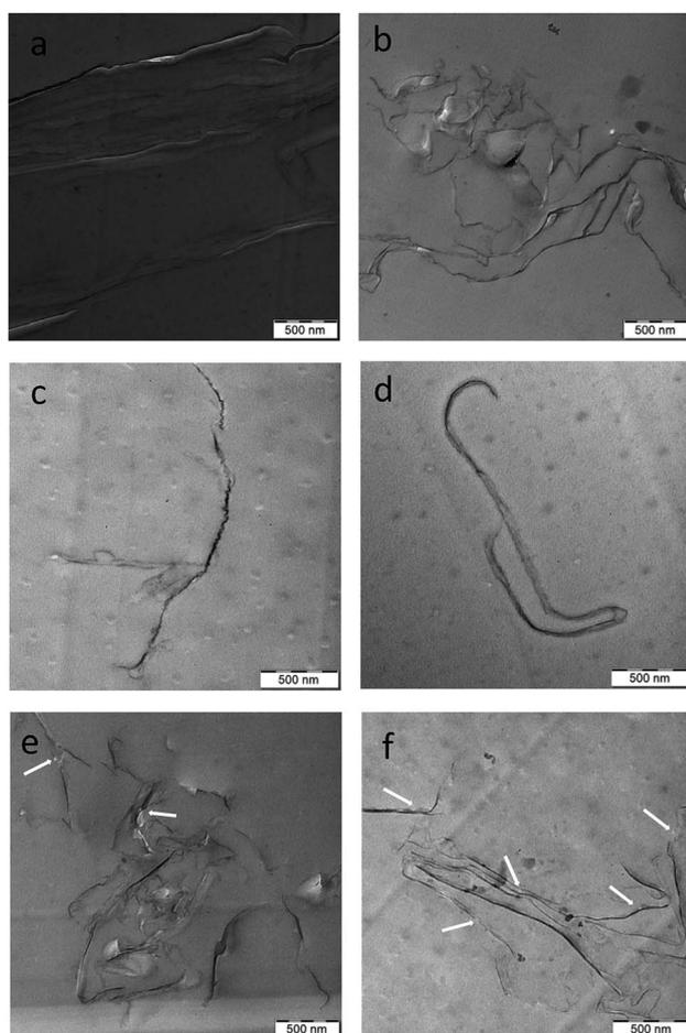
Fig. 3 TEM images of lamellar arrays formed in the epoxy containing (a) GO-*g*-ATBN<sub>plane</sub> (b) GO-*g*-ATBN<sub>edge</sub> (c) GO-*g*-ATBN<sub>plane</sub>+BA (d) GO-*g*-ATBN<sub>plane</sub> + 5% ATBN (e) GO-*g*-ATBN<sub>edge</sub> + 5% ATBN (f) GO-*g*-ATBN<sub>plane</sub>+BA + 5% ATBN; white arrows show the examples of ATBN domains.
