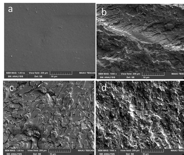
Fig. 7 SEM images of the fracture surfaces of the samples broken by a impact hammer (a) epoxy (b) Ep. + 0.2GO-g-ATBN<sub>plane</sub> (c) Ep. + 0.2GOred + 5ATBN (d) Ep. + 0.2GO + 5ATBN.
