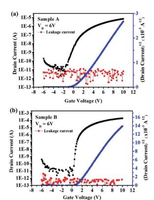
Fig. 3 Measured transfer characteristics and measured leakage current of (a) sample A and (b) sample B, with different dielectric layer.
