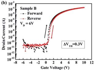
Fig. 5 Hysteresis of transfer characteristics of (a) samples A and (b) B, in which sweep range of gate voltage was -6 V from 10 V.
