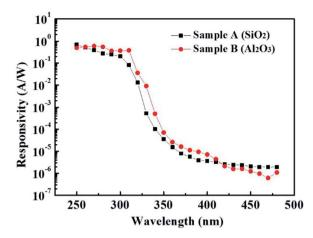
Fig. 7 The responsivity of sample A and sample B were measured at various wavelength and VGS of -5 V.
