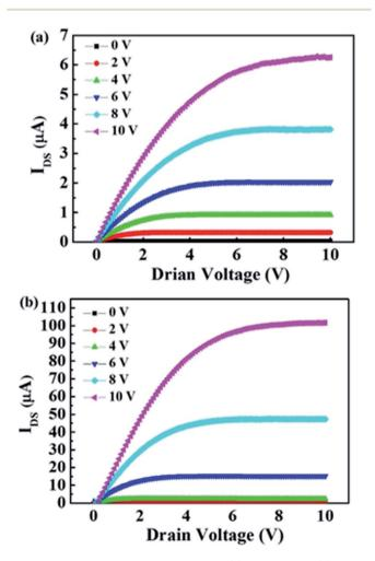
**Fig. 4** Measured output characteristics of (a) sample A and (b) sample B, with different dielectric layer.
