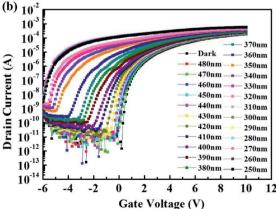
Fig. 6 Transfer characteristics of (a) sample A and (b) sample B measure in the dark condition and under illumination with various light wavelength (480 nm to 250 nm).
