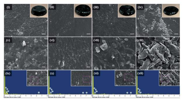
Fig. 6 SEM images of freeze-dried hydrogels: (i) PAA/PPy<sub>5</sub>-Fe; (ii) PAA/PPy<sub>10</sub>-Fe; (iii) PAA/PPy<sub>15</sub>-Fe; and (iv) PAA/PPy<sub>20</sub>-Fe hydrogels at magnification of  $\times$ 500, (v-viii) at  $\times$ 5000 and the EDX spectrum of hydrogels (ix-xii). Scale bars are (i-iv) 20  $\mu$ m and (v-viii) 2  $\mu$ m.
