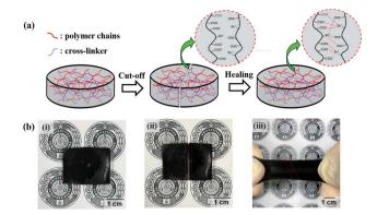
Fig. 2 (a) Illustration of self-healing processes of PAA/PPy-Fe hydrogels *via* ionic interaction and (b) photographs of PAA/PPy-Fe hydrogels in the condition of: (i) initial; (ii) cut-off; and (iii) healed hydrogel under stretching.
