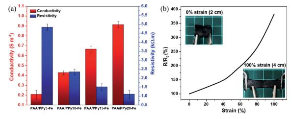
Fig. 8 (a) The electroconductivity and resistivity of PAA/PPy–Fe hydrogels with various concentration of pyrrole and (b) resistance ratio–strain curve of PAA/PPy<sub>20</sub>–Fe hydrogel (the inserted photos are the strain at 0 and 100%).
