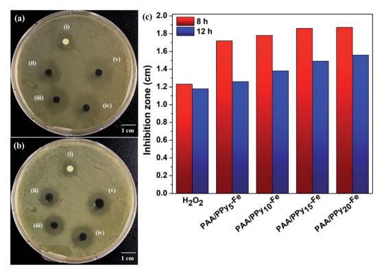
Fig. 7 Antibacterial activity of hydrogels: (i)  $H_2O_2$ ; (ii)  $PAA/PPy_5-Fe$ ; (iii)  $PAA/PPy_{10}-Fe$ ; (iv)  $PAA/PPy_{15}-Fe$ ; and (v)  $PAA/PPy_{20}-Fe$  on *E. coli* bacterial incubated at 37 °C for: (a) 8 h; (b) 12 h and (c) zone of inhibition of PAA/PPy-Fe hydrogels with different composition.
