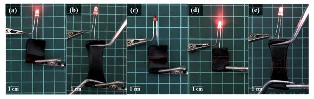
Fig. 9 Photographs of PAA/PPy–Fe hydrogel conducting electricity in an electrical circuit, (a) original; (b) stretched; (c) cut-off; (d) healed; and (e) healed and stretched hydrogel.
