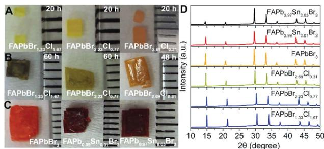
Fig. 1 Photographs of  $\text{FAPbBr}_{3-x}\text{Cl}_x$  (A) based perovskites with a total synthesis time of 20 hours and (B) with a total synthesis time > 48 hours showing a degradation of the surface with increased synthesis time. (C) Photographs of  $\text{FAPb}_{1-x}\text{Sn}_x\text{Br}_3$  based perovskites. (D) Powder XRD spectra of FA based perovskites with different halide and metal compositions.
