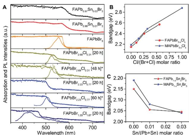
**Fig. 2** Absorption and PL spectra for (A) FA based perovskites with mixed halides or mixed metals. \*Absorption and PL spectra collected for samples with degraded surface (total synthesis time > 48 hours). Band gap of (B) mixed Br/Cl perovskites and (C) mixed Pb/Sn perovskites extrapolated from Tauc plots.
