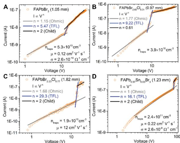
**Fig. 3**  $I$ - $V$  curves of (A)  $\text{FAPbBr}_3$ , (B)  $\text{FAPbBr}_{2.69}\text{Cl}_{0.31}$ , (C)  $\text{FAPbBr}_{2.23}\text{Cl}_{0.77}$ , and (D)  $\text{FAPb}_{0.97}\text{Sn}_{0.03}\text{Br}_3$  perovskite single crystals with regions corresponding to SCLC theory. The crystal thickness is given in the parenthesis and the conductivities are calculated from the ohmic regime, the trap densities are calculated from the TFL and the mobilities are determined from the Child's regime.
