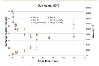
Fig. 3 Oak bio-oils 80  $^{\circ}$ C aging.
