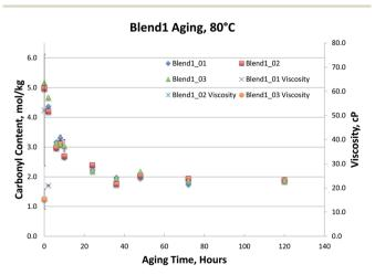
Fig. 1 Blend1 bio-oils 80 °C aging.
