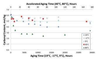
Fig. 8 Accelerated aging vs. long-term storage: carbonyl contents for Oak\_01 Bio-oil.
