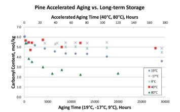
Fig. 9 Accelerated aging vs. long-term storage: carbonyl contents for Pine\_01 bio-oil.
