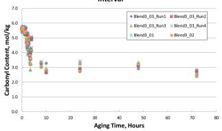
Fig. 10 Fifteen-minute sampling of Blend3 bio-oils aged at 80 °C.
