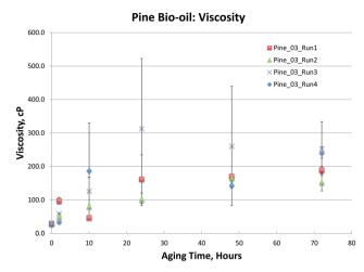
Fig. 5 Viscosity of Pine bio-oils aged at 80 °C.
