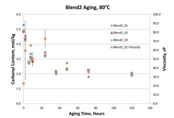
Fig. 2 Blend2 bio-oils 80 °C aging
