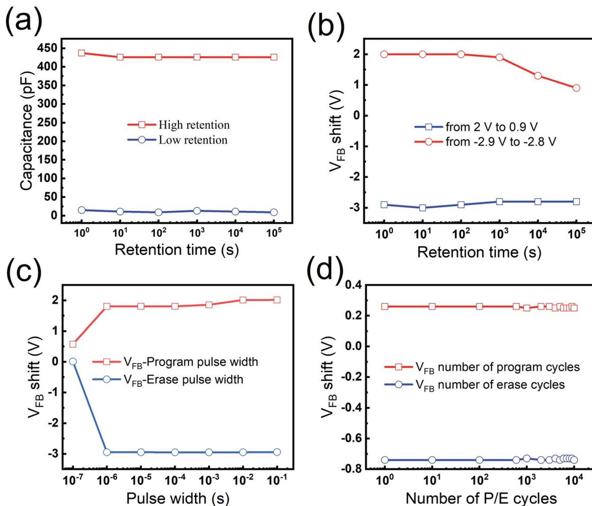
Fig. 4 (a) The high and low capacitances of the memory device based on the single GHO layer and (b) the long-term retention characteristics of the V<sub>FB</sub> shift; (c) the program/erase characteristics of the MGOS device and (d) the endurance characteristic of the MGOS device at room temperature.
