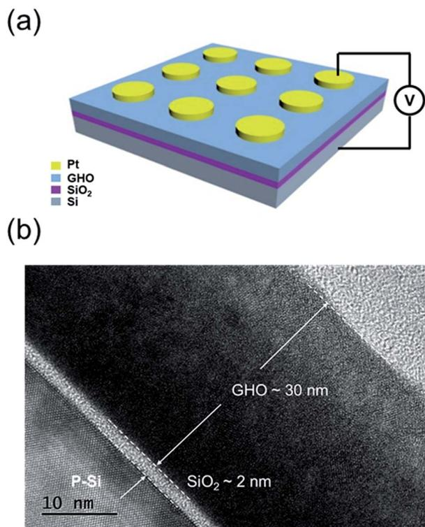
Fig. 1 (a) A schematic of the MGOS device structure and (b) the cross-sectional HRTEM image for a single Gd-doped HfO<sub>2</sub> film.
