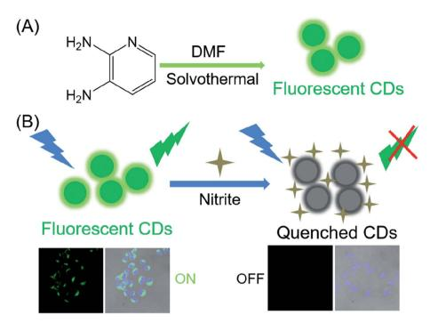
Scheme 1 (A) Schematic route of the carbon dots using 2,3-diamino pyridine precursors; (B) schematic illustration of fabricated CDs for NO<sub>2</sub><sup>-</sup> detection.
