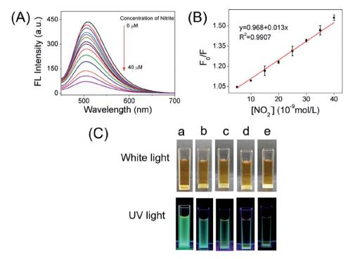
Fig. 4 (A) The fluorescence spectra of the as-prepared CDs by gradual addition of different amounts of  $NO_2^-$  (from top to bottom, respectively). (B) The correlation between fluorescence intensity and  $NO_2^-$  ions at the various concentrations of 5–40 nM. (C) Photographs of the corresponding samples (0.2 mg mL<sup>-1</sup>) under daylight and UV light (a: 0 μM  $NO_2^-$ ; b: 0.02 μM  $NO_2^-$ ; c: 0.1 μM  $NO_2^-$ ; d: 2 μM  $NO_2^-$ ; e: 10 μM  $NO_2^-$ ).
