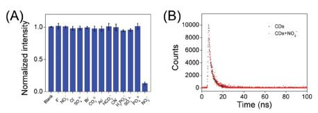
Fig. 5 (A) The normalized fluorescence quenching efficiency of the CDs after addition of multiple interfering ions. (B) Lifetimes of steady-state fluorescence of CDs and CDs + nitrite ions (40 nM).
