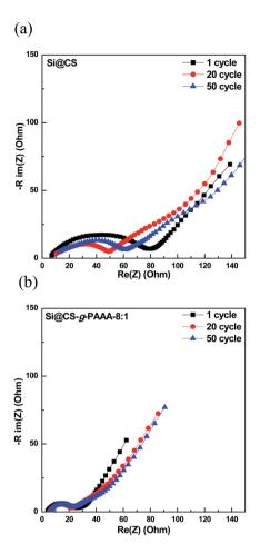
Fig. 6 Electrochemical impedance spectroscopy graphs of (a) Si@CS after 1 cycle, 20 cycles and 50 cycles, and (b) Si@CS-g-PAAA-8:1 binder electrode after 1 cycle, 20 cycles and 50 cycles.
