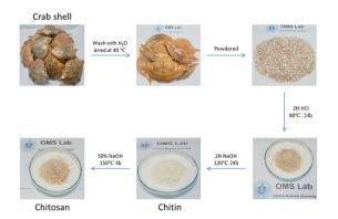
Fig. 3 Procedure for chitosan extraction from crab shell.
