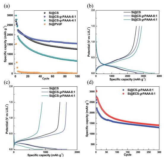
Fig. 5 (a) Specific capacity, (b) voltage profiles of the formation cycle (0.1C), (c) voltage profiles at 50 cycles (0.5C) of the Si@CS (black circle), Si@CS-g-PAAA-8:1 (blue circle), Si@CS-g-PAAA-4:1 (dark cyan circle) and Si@PVdF (orange circle) electrodes, and (d) specific capacity of Si@CS-g-PAAA-8:1 (blue circle) and Si@ECS-g-PAAA-8:1 (red circle).
