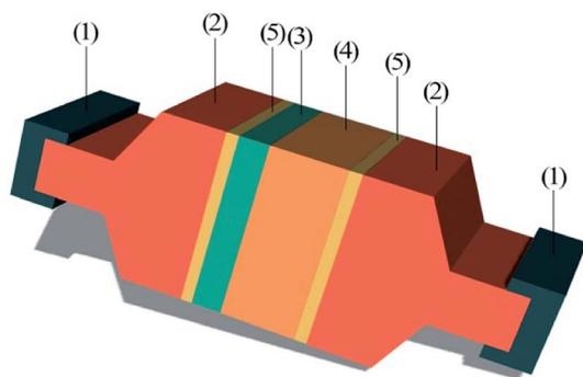
Fig. 8 Schematic diagram of the bonded sample prepared for tensile test: (1) fixtures, (2) extension rods, (3) Al sheet, (4) PUEE sheet, and (5) epoxy glue.
