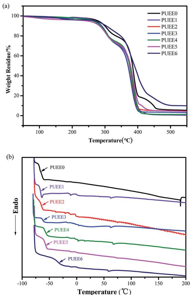
Fig. 4 (a) TGA and (b) DSC curves of the PUEEs in a nitrogen atmosphere at the heating rates of 10 °C min<sup>-1</sup> and 5 °C min<sup>-1</sup>, respectively.
