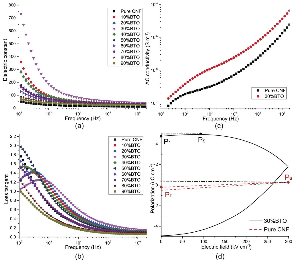
Fig. 4 Dielectric properties of CNF/BTO nanocomposite films. The influence of frequency and filler content on the (a) dielectric constant, (b) dielectric loss, and (c) AC conductivity (d)  $P$ - $E$  hysteresis curves of CNF/BTO nanocomposites.
