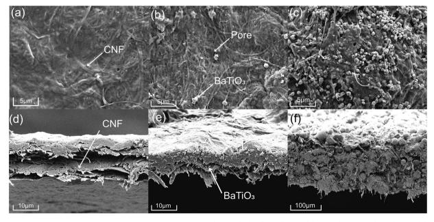
Fig. 2 Surface and cross-section FE-SEM micrographs of pure CNF (a and d), CNF/BTO (30 wt%) (b and e) and CNF/BTO (90 wt%) (c and f) composite films.
