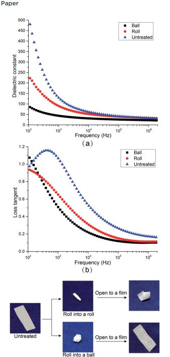
Fig. 5 The influences of rolling treatments on (a) dielectric constant and (b) loss tangent of CNF/BTO nanocomposite films.
