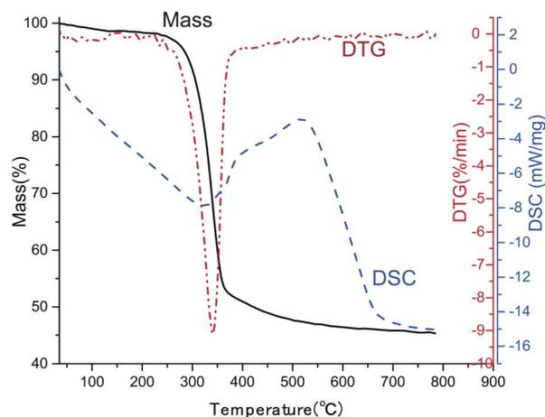
Fig. 6 TGA-DSC curves of CNF/BTO (30 wt%) nanocomposite film.
