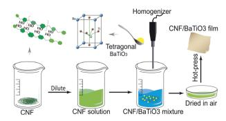
Fig. 1 Preparation of CNF/BTO nanocomposite films.
