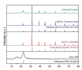
Fig. 3 XRD patterns of pure CNF, untreated BTO, thermally treated BTO, and CNF/BTO (30 wt%) nanocomposite films.
