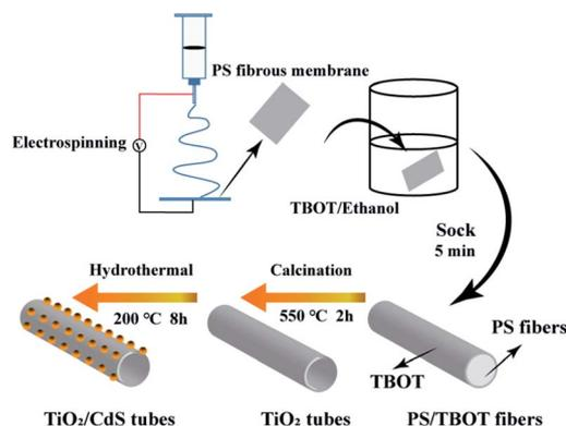
Fig. 1 An illustration of the formation mechanism of the TiO<sub>2</sub>/CdS nanotubes.
