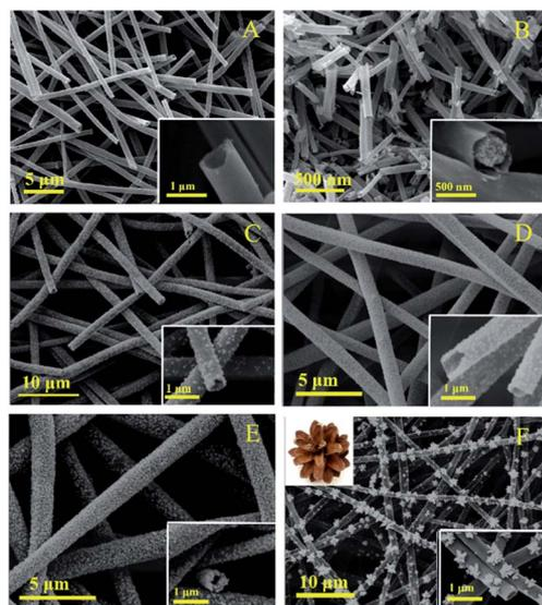
Fig. 3 The SEM images of the samples: (A) TiO<sub>2</sub> nanotubes, (B) core-shell structure TiO<sub>2</sub> nanotubes, (C) TC1 nanotubes, (D) TC2 nanotubes, (E) TC3 nanotubes and (F) TC4 nanotubes.
