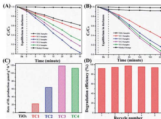
Fig. 8 Degradation rates of as-prepared photocatalysts under the UV-light (A); degradation rates of as-prepared photocatalysts under the visible light (B); the rate of  $\text{H}_2$  evolution on  $\text{TiO}_2/\text{CdS}$  nanotubes under visible light (C); the repeatability tests studied on the TC3 nanotubes for five recycles (D).
