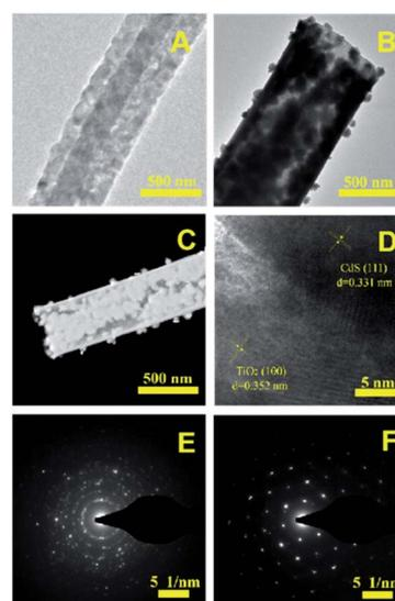
Fig. 4 The TEM image of TiO<sub>2</sub> nanotubes (A) and TC3 nanotubes (B), the STEM image of TC3 nanotubes (C) and the HRTEM of TC3 nanotubes (D), the SAED pattern of the TC3 (E) and the CdS Nps of the surface of TC3 (F).
