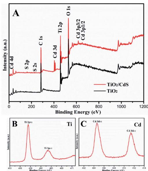
Fig. 5 The XPS spectra of the TiO<sub>2</sub> and TC3 nanotubes: full spectrum of the sample (A), the Ti 2p spectrum (B) and Cd 3d spectrum (C).
