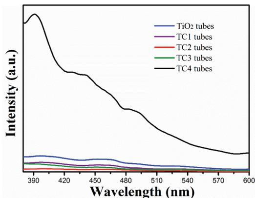
Fig. 7 The photoluminescence spectra of the as-prepared photocatalysts.
