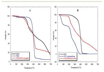
Fig. 6 TGA thermograms of (A) Mox, PEG and PEG-Mox conjugate, (B) molecular PCL, PCL NPs and PCL(PEG-Mox) NPs.
