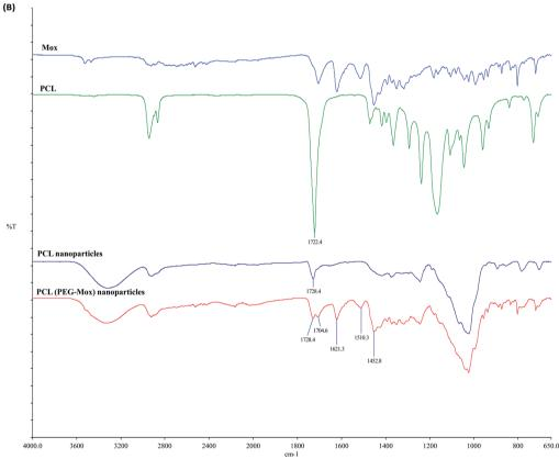
Fig. 3 FTIR spectra of (A) Mox, PEG and PEG-Mox conjugate. (B) Mox, PCL, PCL NPs, and PCL-Mox NPs.
