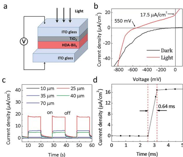
Fig. 3 (a) Schematic diagram of the (HDA-BiI<sub>5</sub>)-based solar device. (b)  $J$ - $V$  curves in dark and under sunlight simulator illumination at room temperature. (c) Zero-voltage photocurrent density with the variation of the HDA-BiI<sub>5</sub> film thickness following on-off sunlight simulator illumination. (d) Response time of (HDA-BiI<sub>5</sub>)-based solar device.
