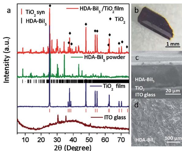
Fig. 1 (a) Comparison of XRD patterns: HDA-BiI<sub>5</sub> thin-film deposited on ITO/TiO<sub>2</sub> substrate (red), HDA-BiI<sub>5</sub> powder (green), TiO<sub>2</sub> thin-film (blue) and pure ITO glass substrate (wine). (b) Optical photograph of HDA-BiI<sub>5</sub> single crystal. (c and d) Cross-sectional and surface SEM images of the ITO/TiO<sub>2</sub>/HDA-BiI<sub>5</sub> hybrid film.
