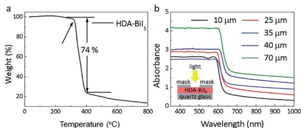
Fig. 2 (a) TGA data for HDA-BiI<sub>5</sub> crystals. (b) UV-Vis absorption spectra of HAD-BiI<sub>5</sub> films with various thicknesses. The inset schematically shows the measurement setup.
