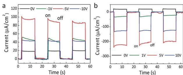
Fig. 4 The  $J$ - $T$  curves of (HDA-BiI<sub>5</sub>)-based solar device after negative (a) and positive (b) poling processes under sunlight simulator illumination.
