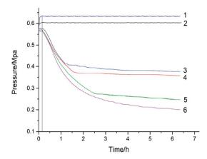
Fig. 3 Pressure *versus* time for cinnamaldehyde,  $1-N_2$ , 353 K;  $2-N_2$ , 308 K;  $3-O_2$ , 308 K;  $4-O_2$ , 318 K;  $5-O_2$ , 328 K;  $6-O_2$ , 338 K.
