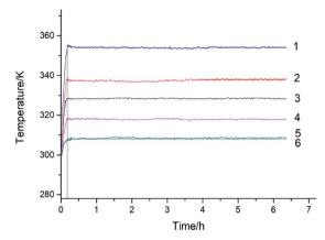
Fig. 4 Temperature *versus* time for cinnamaldehyde,  $1-N_2$ , 353 K;  $2-O_2$ , 338 K;  $3-O_2$ , 328 K;  $4-O_2$ , 318 K;  $5-O_2$ , 308 K;  $6-N_2$ , 308 K.
