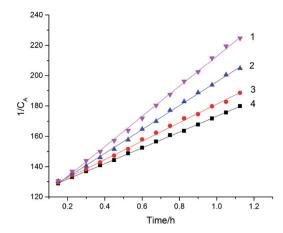
Fig. 5 Plots of  $(1/C_A)$  versus time at different temperatures, 1-338 K; 2-328 K; 3-318 K; 4-308 K.
