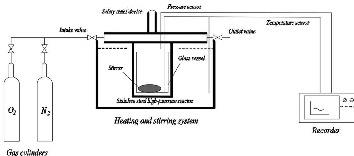
Fig. 1 Experimental installation of the cinnamaldehyde oxidation reaction.
