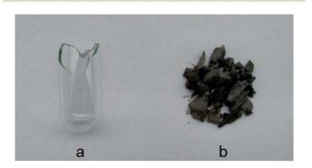
Fig. 11 The aftermath of cinnamaldehyde oxidation (a) round bottom flask (b) broken flask after explosion.
