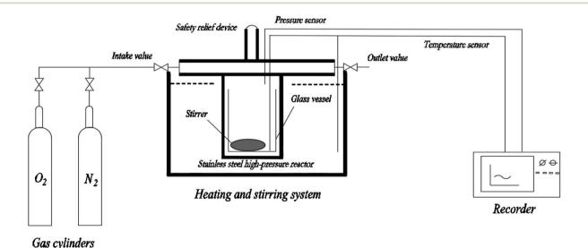
Fig. 1 Experimental installation of the cinnamaldehyde oxidation reaction.
