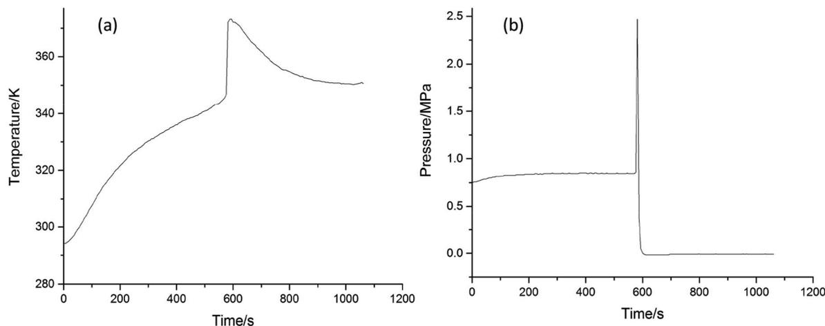
Fig. 9 Explosion studies of cinnamaldehyde oxidation (a) temperature versus time (b) pressure versus time.
