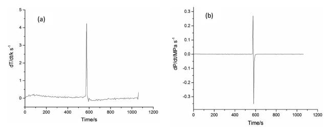
Fig. 10 Explosion of cinnamaldehyde oxidation (a) dT/dt versus time (b) dP/dt versus time.
