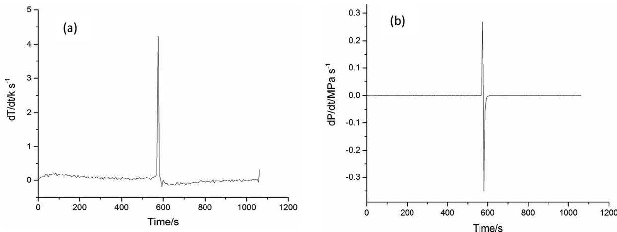
Fig. 10 Explosion of cinnamaldehyde oxidation (a)  $dT/dt$  versus time (b)  $dP/dt$  versus time.
