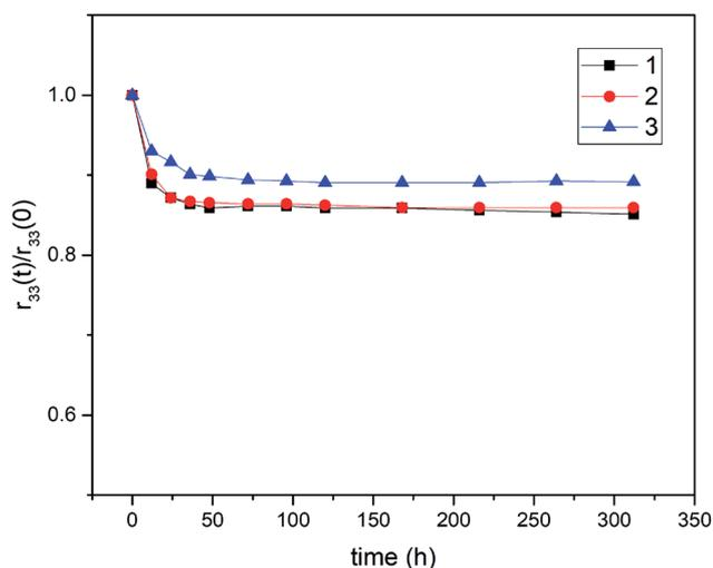
Fig. 5 Long-term stability of the EO polymer films at 80 °C for 300 h.
