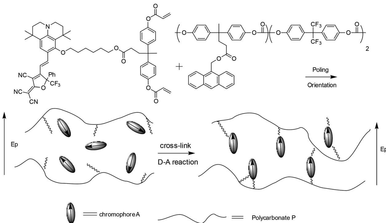
Scheme 3 The crosslinking process of the EO polymers.
