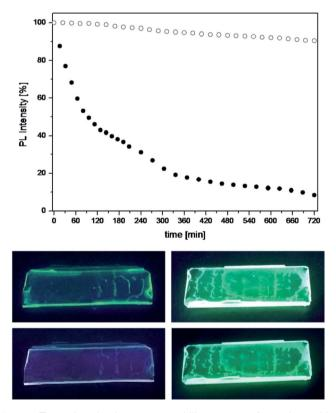
Fig. 4 Top: photoluminescence stability tests performed on thin polymer films doped with the free complex 2 (black circles) and with silica particles embedding the complex (white circles); irradiation wavelength = 450 nm; detection wavelength = 520 nm. Bottom: photographs of the 2-doped (left) and the 2S-doped PMMA films (right), under UV light (365 nm), before (top pictures) and after (bottom pictures) the irradiation tests.
