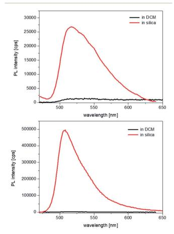
Fig. 3 Emission spectra of the complexes 1 (top) and 2 (bottom) from  $4\times10^{-6}$  M dichloromethane solutions (black lines), compared with equimolar suspensions of the host–guest silica systems in water. All spectra were recorded at  $\lambda_{\text{exc}}=450$  nm, with both excitation and emission slits set at 5 nm.
