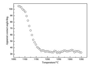
Fig. 1 The wetting angle of Zr–Cu alloy/SiC ceramic changes with temperature.
