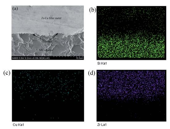
Fig. 5 Interfacial microstructure of Zr-Cu alloy/SiC ceramic after wetting at 1200 °C for 1200 s; (a) XRD of the reaction interface; (b) the distribution of Si element; (c) the distribution of Cu element; (d) the distribution of Zr element.
