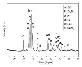
Fig. 6 XRD patterns of the interface of the Zr-Cu alloy/SiC ceramic.
