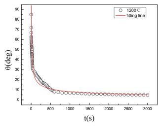
Fig. 3 The apparent contact angle of Zr–Cu alloy/SiC ceramic system changes with heat preservation time during wetting at 1200  $^{\circ}$ C.
