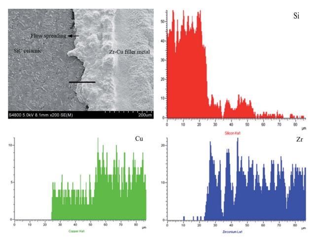
Fig. 4 Precursor film effect and EDS analysis of Zr-Cu/SiC after wetting at 1200 °C for 1200 s.
