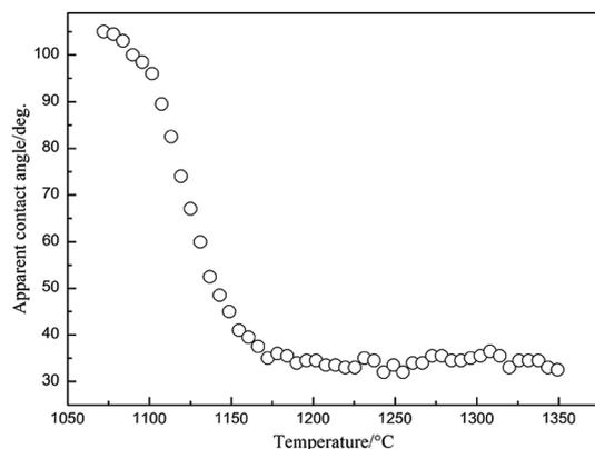
Fig. 1 The wetting angle of Zr–Cu alloy/SiC ceramic changes with temperature.
