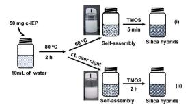
Fig. 2 Schematic representation of self-assembly and silica hybridization of c-iEP in water (inset photographs: aqueous dispersions self-assembled from c-iEP at 60 °C (i) and at room temperature (ii)).
