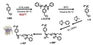
Scheme 1 Synthetic route of comb-like block copolymers c-iEP.
