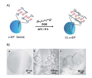
Fig. 7 (A) Schematic representation of the cross-linked polymersome. (B) TEM images of (a) capsule CL-iEP, (b and c)  $SiO_2$ @CL-iEP.
