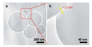
Fig. 4 TEM images of self-assemblies of c-iEP. (a) Low magnification. (b) Magnified image of the red box area in (a).
