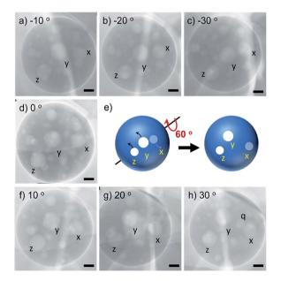
Fig. 5 TEM images of a larger vesicle self-assembled from c-iEP observed by titling the grid from -30 to  $30^{\circ}$  (c  $\rightarrow$  b  $\rightarrow$  a  $\rightarrow$  d  $\rightarrow$  f  $\rightarrow$  g  $\rightarrow$  h) and (e) schematic image after tilting  $60^{\circ}$  from -30 to  $30^{\circ}$ . Scale bar was 100 nm.
