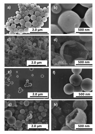
Fig. 3 SEM images of self-assembled entities from c-iEP and c-iPE@silica hybrids. ((a, b) and (e, f)) c-iEP, ((c, d) and (g, h)) c-iEP@SiO<sub>2</sub>; (a-d) formed at room temperature; (e-h) formed at  $60 \, ^{\circ}$ C.
