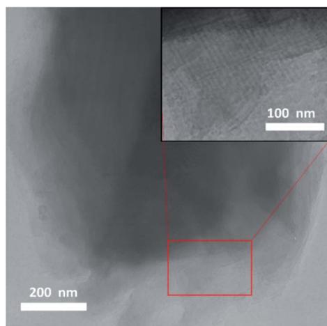
Fig. 11 A fragment of crystal **6** after immersion into water. The lamellar structure originates from hydrolysis–condensation reactions of **6** with water that results first in cracking of the original crystal into plates with subsequent formation of layers of densified titanium oxo-alkoxide material.
