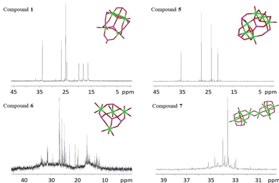
Fig. 12  $^{31}\text{P}$  NMR spectra of compounds 1, 5, 6 and 7. The titanium oxo-cores with phosphorus atoms are inserted in their respective spectrum. Green is titanium, red is oxygen and magenta is phosphorus.
