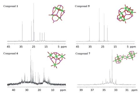
Fig. 12 <sup>31</sup>P NMR spectra of compounds 1, 5, 6 and 7. The titanium oxo-cores with phosphorus atoms are inserted in their respective spectrum. Green is titanium, red is oxygen and magenta is phosphorus.
