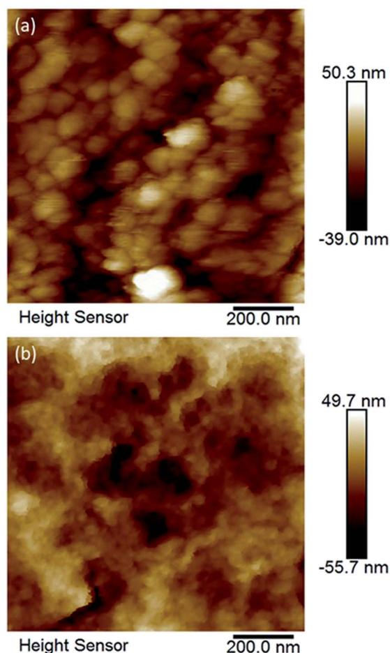
Fig. 8 AFM micrographs of (a) hydrolysed compound **1** (no chelating ligands), and (b) hydrolysed compound **6** (one chelating ligand per titanium atom). Both compounds yielded rather uniform titania nanoparticles which apparently are aggregates of primary anatase nuclei according to TEM.
