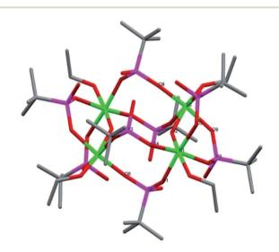
Fig. 3 Molecular structure of compound 3. Green it titanium, red is oxygen, magenta is phosphorous and grey is carbon. The solvating ethanol molecules and hydrogen atoms have been omitted for clarity. Selected bond lengths (Å) and angles (°): Ti1-O2 1.682(4), Ti1-O1 1.959(4), Ti1-O14 1.986(4), Ti1-O4 2.001(4), Ti2-O6 1.767(4), Ti2-O8 1.902(4), Ti2-O7 1.984(4), Ti2-O9 2.007(4) Ti1-O2-Ti2 142.79(19), P5-O1-Ti1 139.4(2).
