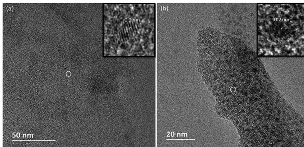
Fig. 10 TEM micrographs of hydrolysis products of **1** and **6**. (a) Anatase particles from the hydrolysis of **1** are visible as dark spots. The insert shows a magnified particle. The lattice fringe distance is 0.2 nm. (b) A crystal fragment of **6**. The dark spots are anatase nuclei of about 2 nm in diameter. The inset shows a magnified particle. The lattice fringe spacing of the particle is 0.2 nm.
