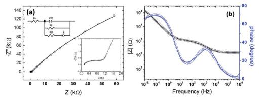
Fig. 7 (a) Nyquist and (b) Bode plots recorded for the photocapacitor device at an applied bias potential of 0.0 V under dark conditions. The symbols (open circle shapes) stand for experimental data; the solid lines are the curves fitted to the electrical circuit model depicted in the inset of (a). The inset shows the high frequency region.
