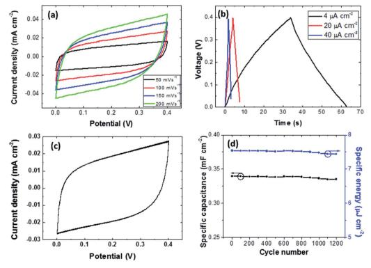
Fig. 6 (a) Cyclic voltammetry curves at different scan rates in darkness. (b) Galvanostatic charge—discharge curves at different current densities. (c) Cyclic voltammograms measured at 100 mV s<sup>-1</sup> from 1200 cycles. (d) Specific capacitance (black circles) and specific energy (blue circles) values obtained from the CV curves of the photocapacitor.
