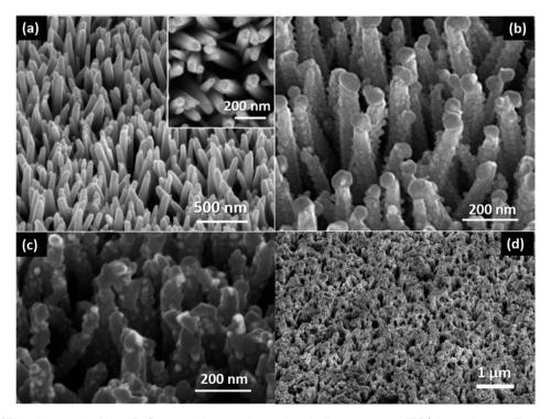
Fig. 3 (a) Tilted FESEM micrograph of bare ZnO nanorod arrays electrochemically grown on a FTO/glass substrate. The inset of (a) shows the high magnification top view image of the ZnO nanorod arrays. (b) Tilted FESEM micrograph of the ZnO nanorod arrays after decoration with  $Ag_2S$  QDs. (c) Tilted FESEM image of ZnS covering the  $Ag_2S$  QDs@/ZnO NR nanostructure. (d) Tilted FESEM micrograph showing the PEDOT layer grown on the ZnS@Ag\_S QDs@ZnO NR nanostructure.
