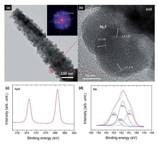
Fig. 4 (a) HRTEM image of a single ZnO nanorod decorated with  $Ag_2S$  QDs. The inset shows the FFT pattern. (b) High-magnification HRTEM image of (a) depicting individual  $Ag_2S$  QDs. (c) The  $Ag_2S$  QDs analysis.
