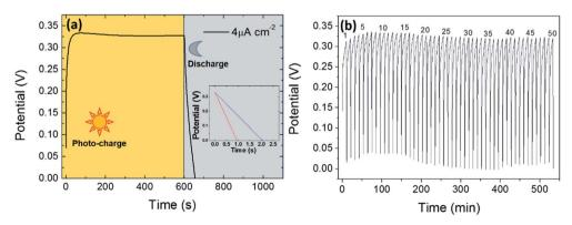
Fig. 8 (a) Photocharge under AM1.5G simulated sunlight (100 mW cm $^{-2}$ ) illumination and galvanostatic discharge at 4  $\mu$ A cm $^{-2}$  in dark conditions (inset shows the galvanostatic discharge at 40  $\mu$ A cm $^{-2}$  (blue line) and 400  $\mu$ A cm $^{-2}$  (red line) current densities). (b) Some cycles of photocharge/galvanostatic discharge at 4  $\mu$ A cm $^{-2}$ . Cycle numbers are indicated.
