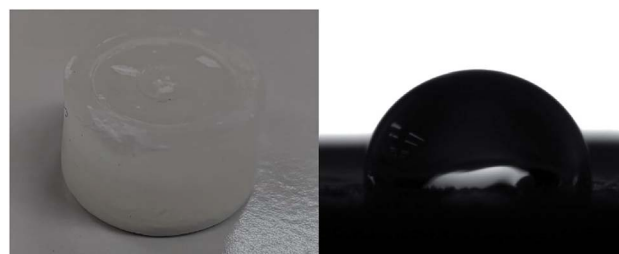
Fig. 2 Picture (a) and contact angle measurement of sample FS4 (b).
