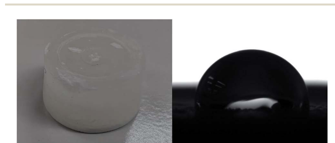
Fig. 2 Picture (a) and contact angle measurement of sample FS4 (b).
