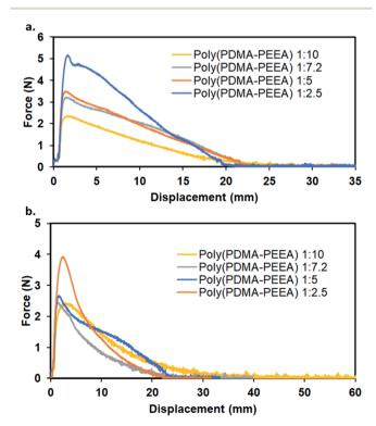
Fig. 3 Mechanical properties of adhesive copolymer, poly(PDMA-PEEA). Force-displacement curves (a) using glass-co-polymer-PTFE and (b) PTFE-co-polymer-PTFE substrates respectively.
