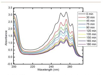
Fig. 9 UV-visible spectra of pyridine showing its degradation with time (10 mg of nanocomposite, 50 ml Py solution (100 ppm), 25  $^{\circ}$ C and pH 7).
