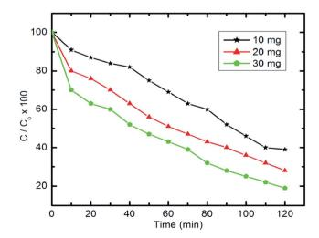
Fig. 13 Effect of photocatalyst dose on pyridine degradation efficiency (50 ml Py solution (100 mg  $l^{-1}$ ), 25 °C and pH 7).
