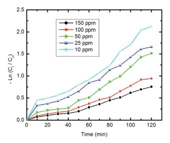
Fig. 11 The first-order kinetics of pyridine degradation (10 mg of composite, 50 ml Py solution, 25  $^{\circ}\text{C}$  and pH 7).
