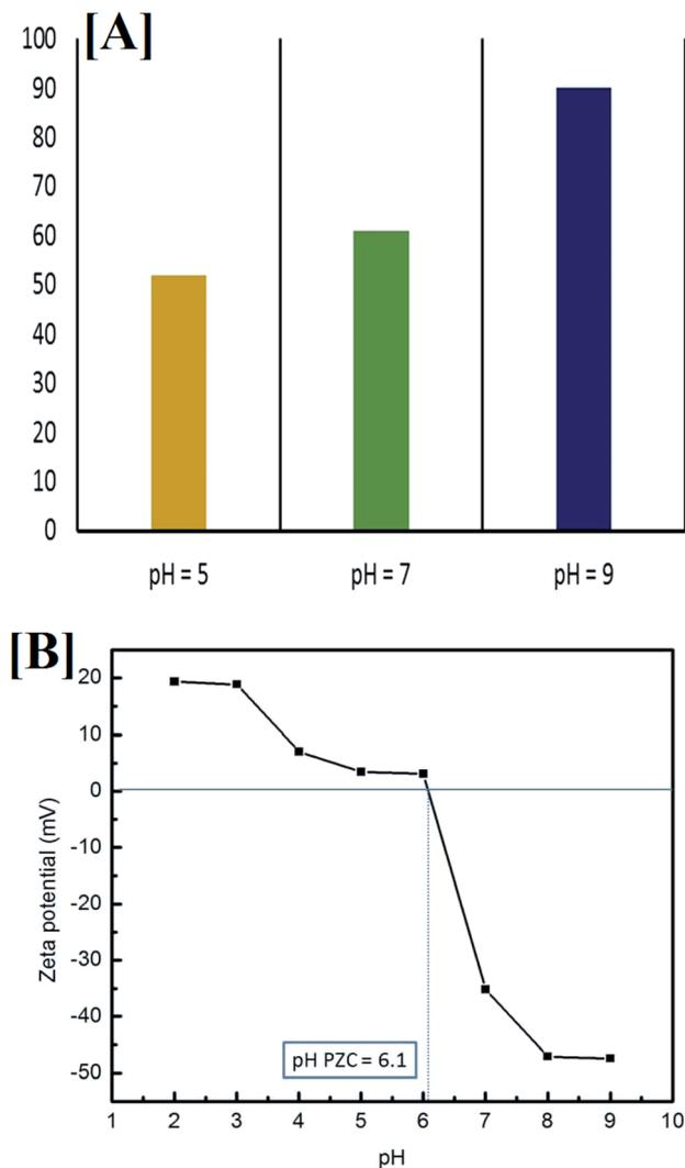
Fig. 14 [A] Influence of initial pH on the removal of pyridine (50 ml pyridine (100 mg l<sup>-1</sup>), 10 mg nanocomposite and 100 min irradiation time) and [B] the point of zero charge (PZC) of Co<sub>x</sub>Ni<sub>1-x</sub>Fe<sub>2</sub>O<sub>4</sub>/SiO<sub>2</sub>/TiO<sub>2</sub>; x = 0.9 at different pH values.
