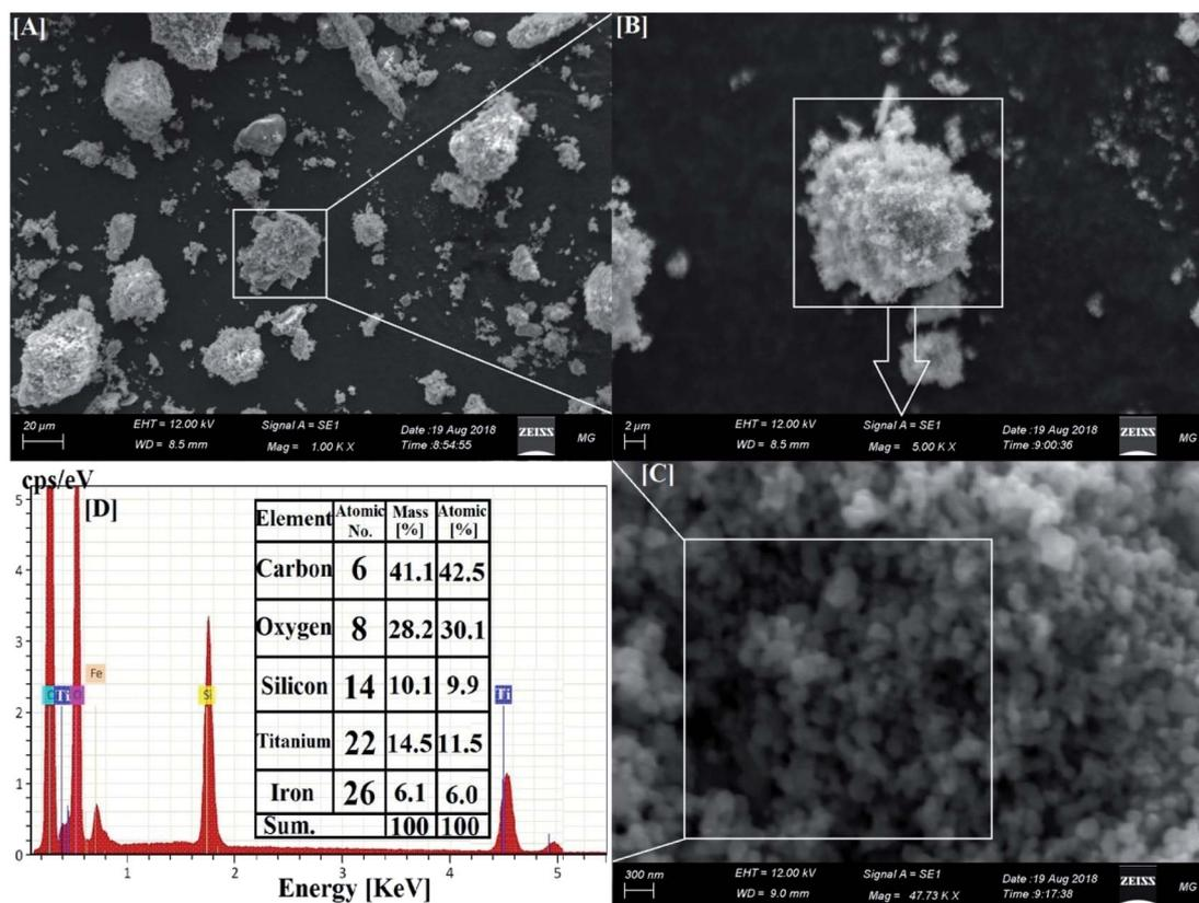
Fig. 2 SEM and corresponding EDX elemental analysis of the synthesized  $\text{Co}_x\text{Ni}_{1-x}\text{Fe}_2\text{O}_4/\text{SiO}_2/\text{TiO}_2$ ;  $x = 0.9$  nanocomposite. [A–C] Different magnifications of the core–multi-shell structure. [D] The corresponding EDX elemental analysis of the synthesized nanocomposite.
