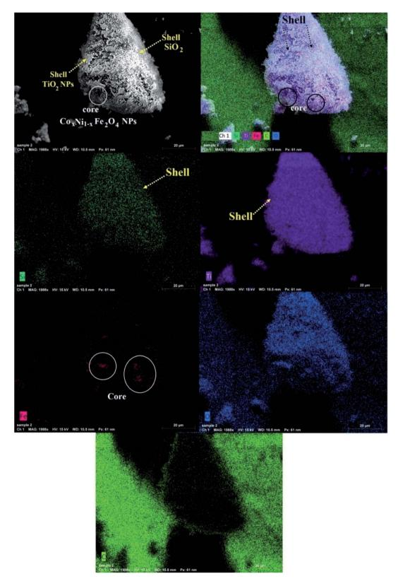
Fig. 3 SEM-EDX elemental mapping of the synthesized  $Co_xNi_{1-x}Fe_2O_4/SiO_2/TiO_2$ ; x=0.9 nanocomposite.
