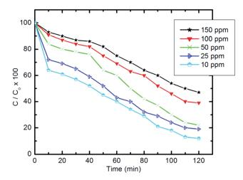
Fig. 10 Effect of initial concentration of pyridine solution on the degradation efficiency (10 mg of composite, 50 ml Py solution, 25  $^{\circ}$ C and pH 7).
