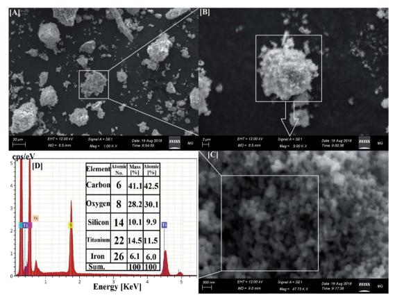
Fig. 2 SEM and corresponding EDX elemental analysis of the synthesized  $Co_xNi_{1-x}Fe_2O_4/SiO_2/TiO_2$ ; x = 0.9 nanocomposite. [A-C] Different magnifications of the core–multi-shell structure. [D] The corresponding EDX elemental analysis of the synthesized nanocomposite.
