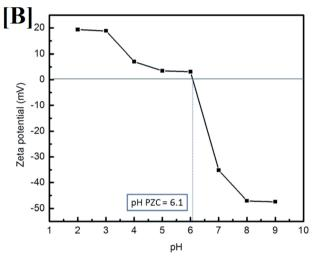
Fig. 14 [A] Influence of initial pH on the removal of pyridine (50 ml pyridine (100 mg l $^{-1}$ ), 10 mg nanocomposite and 100 min irradiation time) and [B] the point of zero charge (PZC) of  $Co_xNi_{1-x}Fe_2O_4/SiO_2/TiO_2$ ; x=0.9 at different pH values.
