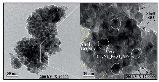
Fig. 1 HRTEM analysis of the prepared  $Co_xNi_{1-x}Fe_2O_4/SiO_2/TiO_2$ ; x=0.9 hybrid nanocomposite concentric structure, where yellow and black arrows display the two shell layers and the white circles represent the core  $Co_xNi_{1-x}Fe_2O_4$ ; x=0.9 NPs.
