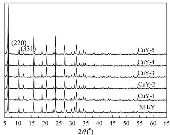
Fig. 1 The XRD patterns of  $\text{NH}_4\text{Y}$  and the CuY catalysts.
