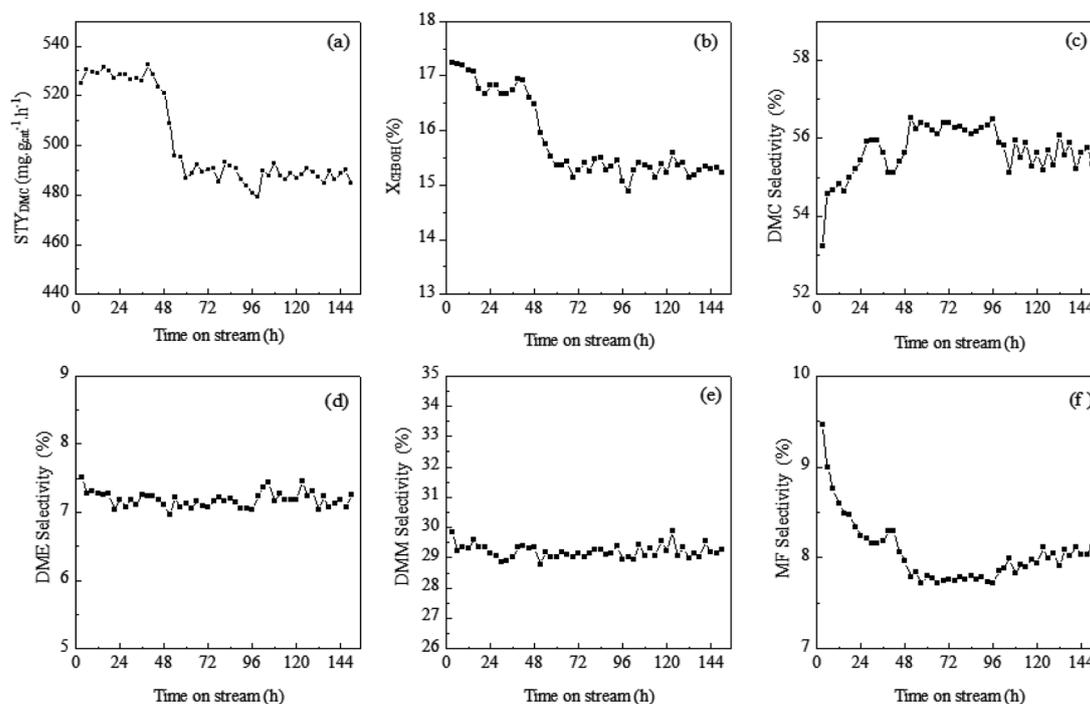
Fig. 6 The long-term catalytic performance of the CuY-5 catalyst. (a)  $STY_{DMC}$ , (b)  $X_{CH_3OH}$ , (c) DMC selectivity, (d) DME selectivity, (e) DMM selectivity, (f) MF selectivity. The testing temperature is  $170 \text{ }^\circ\text{C}$ .
