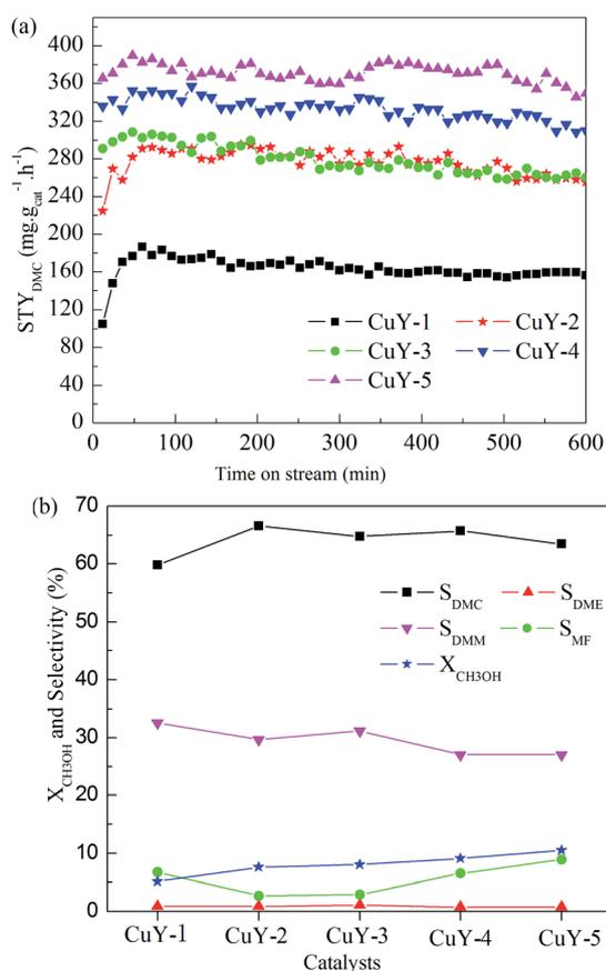
Fig. 4 Catalytic activities of CuY catalysts in the vapor-phase oxidative carbonylation of methanol to DMC at atmospheric pressure. (a) Time-on-stream performance of all CuY catalysts. (b) Selectivity of organic products and X<sub>CH<sub>3</sub>OH</sub>. Testing time and temperature is 10 h and 140 °C respectively.
