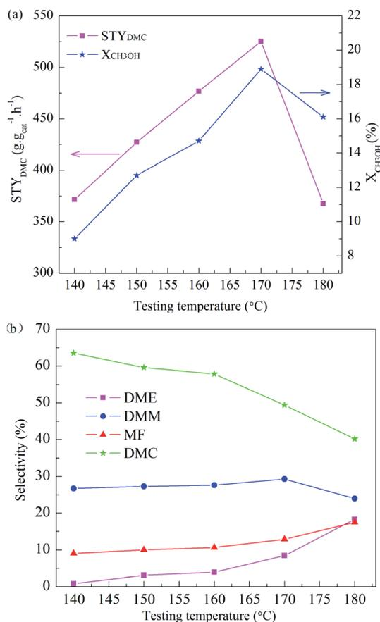
Fig. 5 Catalytic activities of the CuY-5 catalyst with different testing temperature in the vapor-phase oxidative carbonylation of methanol to DMC at atmospheric pressure. (a) STY<sub>DMC</sub> and X<sub>CH<sub>3</sub>OH</sub>, (b) selectivity of organic products. Reaction time is 10 h and the testing temperature is 140 °C, 150 °C, 160 °C, 170 °C, 180 °C respectively.
