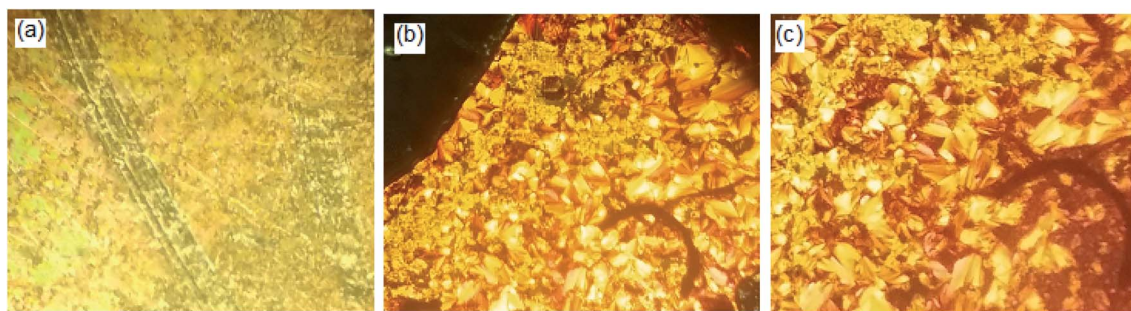
Fig. 3 PLM textures of: (a) the nematic phase of I12 b at 240.0 °C upon cooling; (b) smectic A phase of I16 d at 299.0 °C upon heating; (c) smectic A phase of I16 d at 280.0 °C upon cooling.
