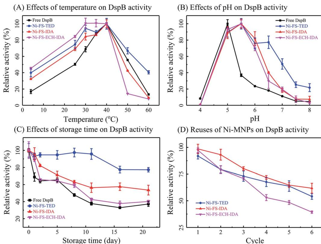
Fig. 6 Enzymatic activity of Ni-MNPs immobilized DspB. Effects of temperature (Panel A), pH (Panel B), storage time (Panel C) and reuses (Panel D) on activities of DspB before and after immobilization on Ni-MNPs.
