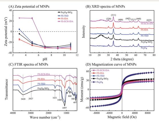
Fig. 3 Characterization of MNPs. Panels (A), zeta potential; Panel (B), XRD spectra; Panel (C), FTIR spectra; Panel (D), magnetization curves.
