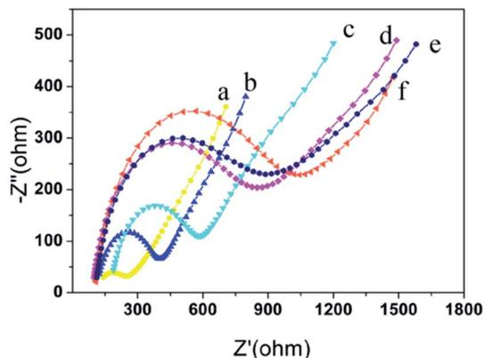
Fig. 4 Nyquist plots of impedance spectra by using different modified electrodes in 5 mM  $[\text{Fe}(\text{CN})_6]^{3-/4-}$ . (a) Bare GCE; (b) Au NPs/IL-MoS<sub>2</sub>/chitosan/GCE; (c) anti-CRP/Au NPs/IL-MoS<sub>2</sub>/chitosan/GCE; (d) BSA/anti-CRP/Au NPs/IL-MoS<sub>2</sub>/chitosan/GCE; (e) CRP/BSA/anti-CRP/Au NPs/IL-MoS<sub>2</sub>/chitosan/GCE; (f) Ir NPs/GO-DN labeled-anti-CRP/CRP/BSA/anti-CRP/Au NPs/IL-MoS<sub>2</sub>/chitosan/GCE.
