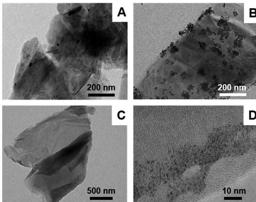
Fig. 2 TEM characterizations of different materials: (A) Au NPs/MoS<sub>2</sub>; (B) Au NPs/IL-MoS<sub>2</sub>; (C) GO-DN; (D) Ir NPs/GO-DN.
