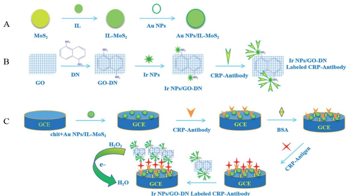
Fig. 1 Flowchart of the preparation of immunosensor.
