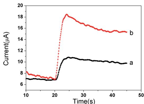
Fig. 3 Comparison of the catalytic effect of (a) GO-DN and (b) Ir NPs/GO-DN to the reduction of 3% H<sub>2</sub>O<sub>2</sub>.
