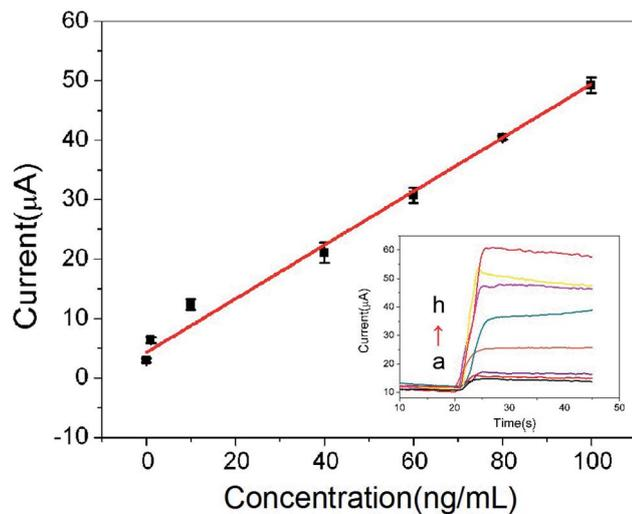
Fig. 6 The calibration curve of the immunosensor (the embedded figure is the  $i-t$  curve response of the sensor to different concentrations of CRP, (a) blank; (b)  $0.01 \text{ ng mL}^{-1}$ ; (c)  $1 \text{ ng mL}^{-1}$ ; (d)  $10 \text{ ng mL}^{-1}$ ; (e)  $40 \text{ ng mL}^{-1}$ ; (f)  $60 \text{ ng mL}^{-1}$ ; (g)  $80 \text{ ng mL}^{-1}$ ; (h)  $100 \text{ ng mL}^{-1}$ ).
