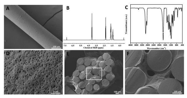
Fig. 2 The physical characterizations of cytokine-loaded PCL-PEG scaffold composite. (A) A representative scanning electron microscopy (SEM) image of PCL; (B and C) analysis of PCL by infrared spectrum (IR) and nuclear magnetic resonance spectroscopy (NMR); (D and E) a representative scanning electron microscopy (SEM) image of PEG and cytokine-loaded PCL-PEG scaffold composite; (F) enlarged view of the scaffold composite.
