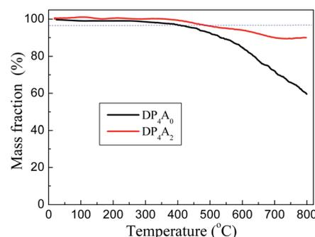
Fig. 4 TGA thermograms of DP<sub>4</sub>A<sub>0</sub> (black) and DP<sub>4</sub>A<sub>2</sub> (red), measured in a nitrogen atmosphere at a heating rate of 10 °C min<sup>-1</sup>.
