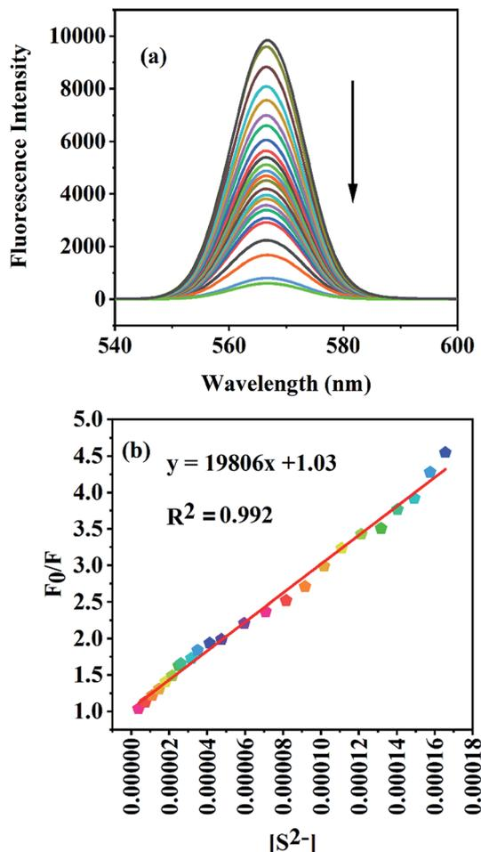
Fig. 5 (a) Fluorescence turn-off response of the GA-AgNPs-Hg(II) ensemble in the presence of an increasing concentration of  $S^{2-}$  [ $3-170 \mu\text{mol L}^{-1}$ ]; (b) the relative fluorescence intensity at 567 nm against  $S^{2-}$ .
