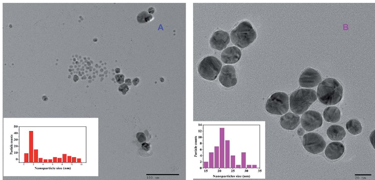
Fig. 3 TEM image of GA-AgNPs alone (A) and GA-AgNPs in the presence of 100 nmol L<sup>-1</sup> Hg(II) ions (B). Insets give the size distribution histogram.
