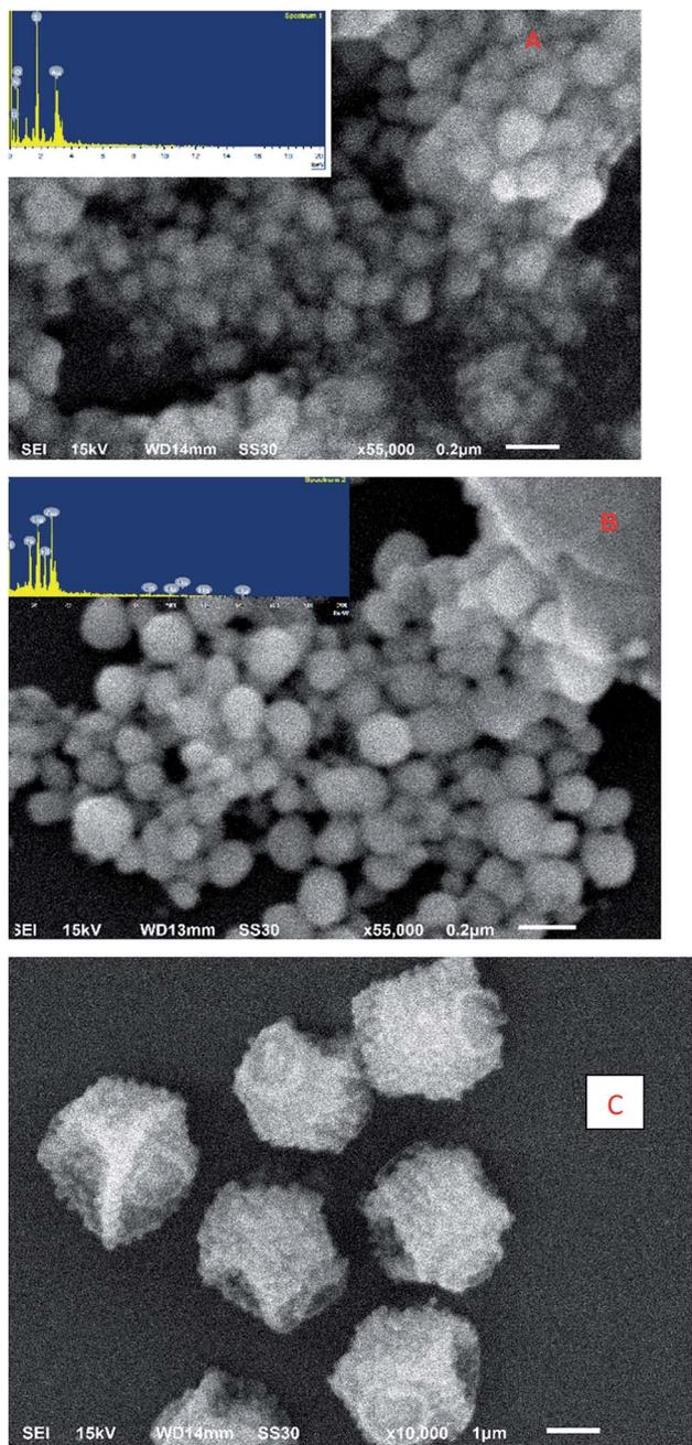
Fig. 2 SEM images of GA-AgNPs (A), GA-AgNPs in the presence of 100 nmol L<sup>-1</sup> Hg(II) (B) and GA-AgNPs in the presence of 100 nmol L<sup>-1</sup> and 30 μmol L<sup>-1</sup> S<sup>2-</sup> ions (C). Insets of (A) and (B) give the EDX image.
