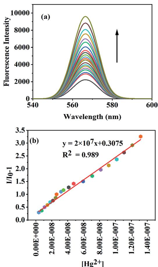
Fig. 4 (a) Fluorescence turn-on response of GA-AgNPs in the presence of an increasing concentration of Hg(II) [3 nmol L<sup>-1</sup> to 13 μmol L<sup>-1</sup>]; (b) calibration curve showing fluorescence enhancement linearity.
