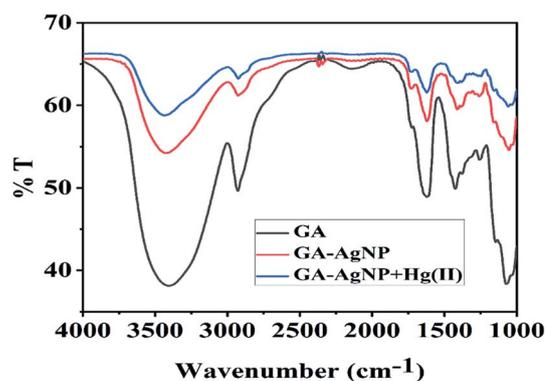
Fig. 1 The FT-IR spectrum of Gum Acacia (GA) (black), GA-capped AgNPs (red), and GA-capped AgNPs in the presence of 100 nmol L<sup>-1</sup> Hg(II) ions (blue).
